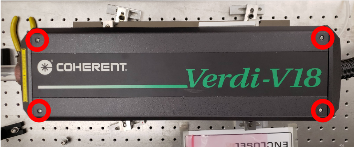
Figure A.2. Coherent Verdi-V18 showing (red circles) which screws need to be removed to slide the cover off.
