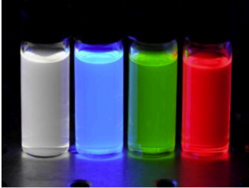
Figure 1.1. CdSe nanocrystals ranging from ultrasmall white light emitting (left) to ~7 nm red emitting (right). These QDs exhibit the size dependence of quantum confinement.
