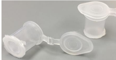
Figure 6.2 Wash buckets used for DRG processing. The tulle ribbon used as “mesh” can be procured easily and affordably from any craft store.
