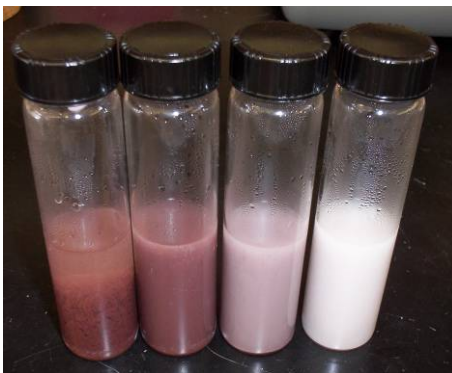
Figure 2.10 Image of Cd-phosphonate reactions. From left to right the reaction times for the vials are: 15, 34, 49, and 62 hours.
