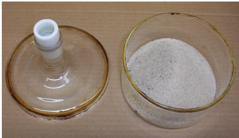
Figure 2.12 Image of the custom-made curing apparatus used when curing films under an inert atmosphere.
