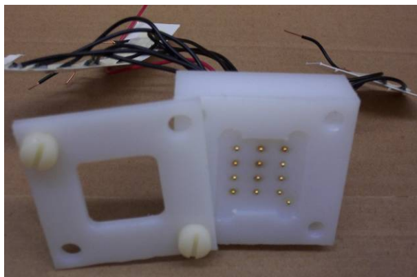
Figure 2.18 Sophisticated plastic holder for the electro-optical analysis of QD-LEDs.
