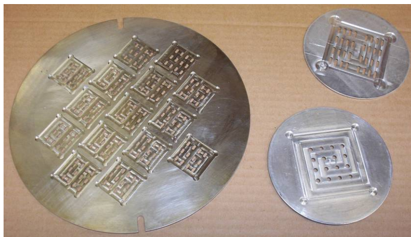
Figure 2.16 Image of evaporator masks fabricated by the Vanderbilt machine shop for use with the Edwards thermal evaporator located in the Rosenthal lab. The largest mask was fabricated with the capacity to be used at the Center for Nanophase Materials Sciences at Oak Ridge National Laboratories.
