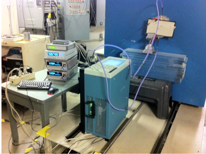
Fig. 30. Broadbeam experimental setup at LBNL. The HEMT is mounted on a high-speed package and placed along the beam line (top of the picture).
