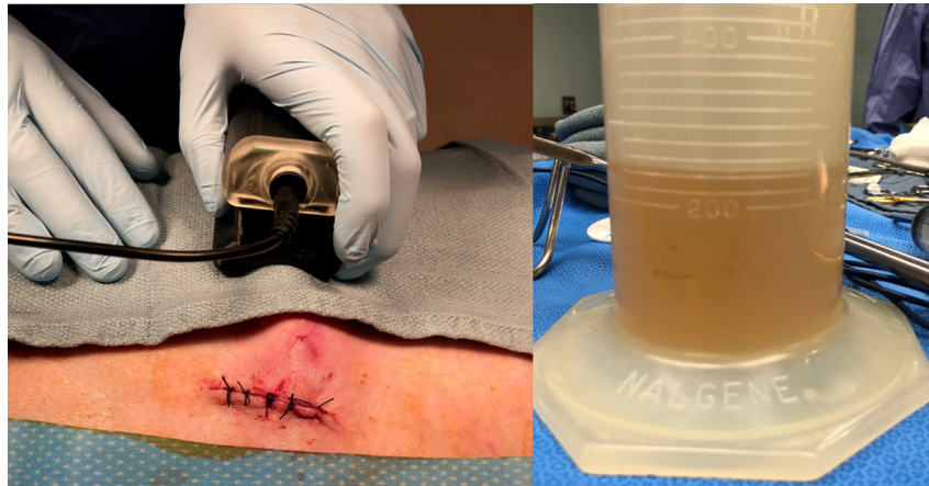
Figure II.55: Left: modified MEC placed over a 2 mm thick fabric actuating the pump; Right: bladder content after 10 minutes actuation.
