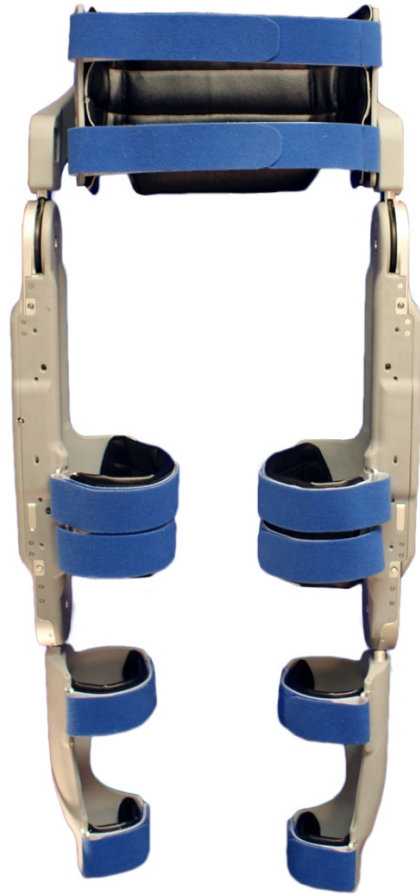
Figure 2-2. Vanderbilt gait restoration orthosis frontal view.
