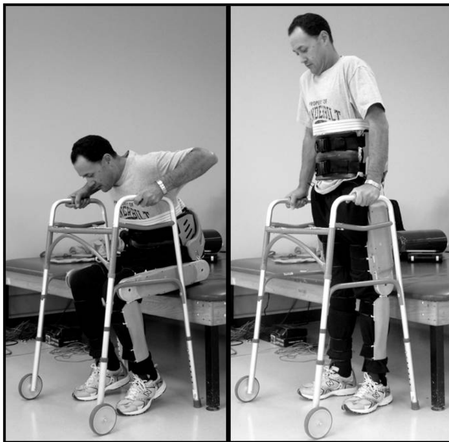
Figure 5-7. Sit-to-stand cooperative control experiment.
