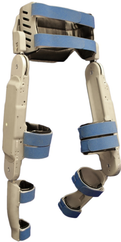
Figure 2-1. Vanderbilt gait restoration orthosis oblique view.
