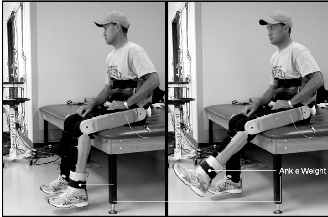
Figure 5-4. Experimental setup for cooperative control of weighted leg lifts.
