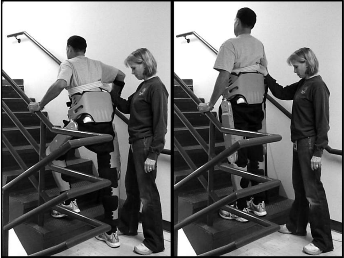
Figure 5-9. Stair ascent cooperative control experiment.
