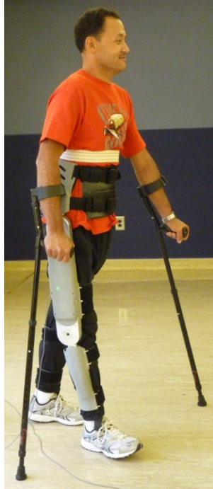
Figure 4-3. T10 complete paraplegic subject wearing Vanderbilt exoskeleton.
