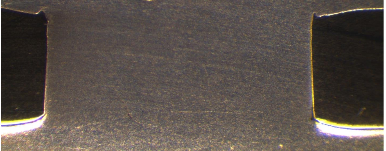
Figure 121: Al-Steel-Al with through hole. 1200 rpm, 5 sec, 8000 N control force. The extruded material from the top and bottom sheets has completely filled the volume of the through hole. There is no observable joint line.
