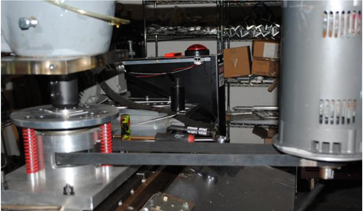
Figure 83: The RAFSSW Device. The motor can be seen mounted in front of the welding machine. During welding the worktable and rotating anvil would raise causing the belt to slip.
