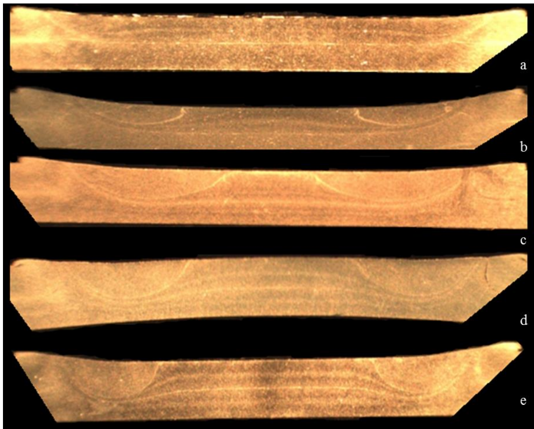
Figure 67: Macrosections of spot welds. Hold parameters: 2 sec dwell, 0.006 in plunge depth, 0.5 ipm plunge rate. a) 750 rpm b) 1000 rpm c) 1250 rpm d) 1500 rpm e) 1750 rpm
