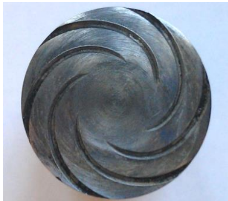
Figure 91: Pinless FSSW tool with a spherically tapered shoulder.
