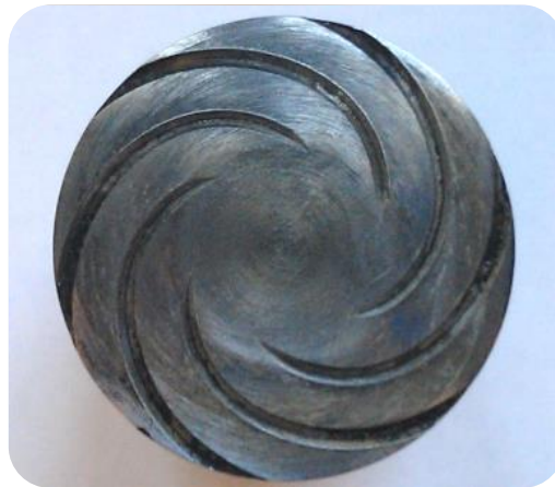
Figure 86: The welding tool and rotating anvil. A spherically tapered (convex) shoulder with scrolling and a 10.2 mm flat ground into the end.
