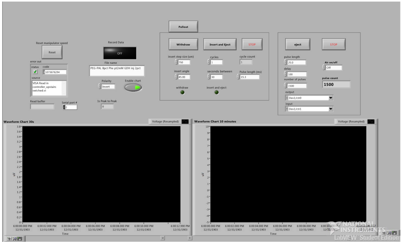
Figure 23. Calorimeter control and recording front panel. Controls micromanipulator and picospritzer, automates sample injection, calibrate pipettes, filters data, and records data.
