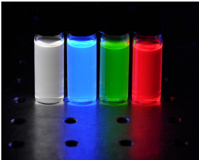
Figure 1.3. CdSe nanocrystals fluorescing under UV excitation ranging in sizes from ultrasmall <2\text{ nm} (left) up to 7\text{ nm} (right), illustrating the size-dependent effects of quantum confinement.
