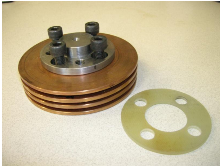
Figure 48, Heat Sink and Thermal Barrier
