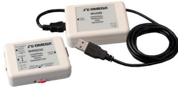
Figure 35, Universal Wireless RS232 to USB Transceiver (Universal, 2010)
