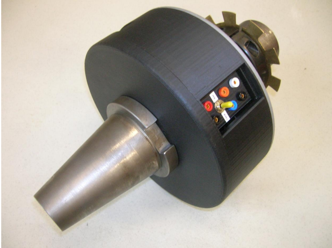
Figure 56, Custom Force Transducer for FSW
