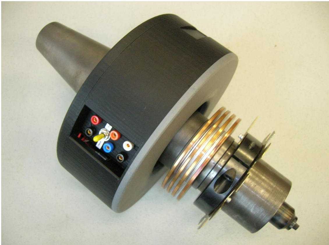
Figure 55, Custom Force Transducer for FSW
