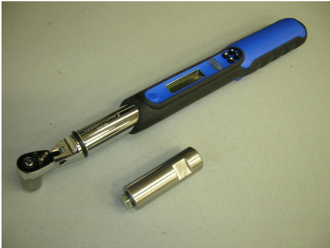
Figure 57, Torque Wrench and Adapter Tool
