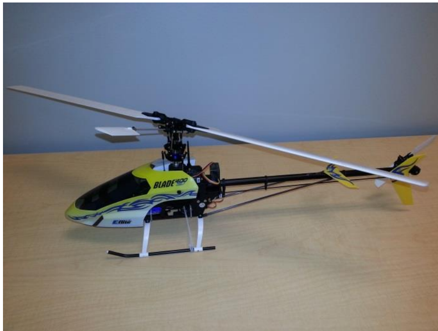
Figure 6.12: RC helicopter used for load/strain data acquisition testing
