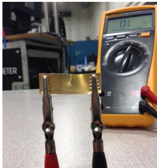
Figure 6.8: Damaged Metal Rubber rectangular test specimen experimental test setup
