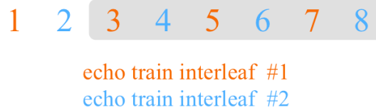
Figure 2.4-1. Echo train interleaves. Echoes shaded with the gray box are included during image analysis.
