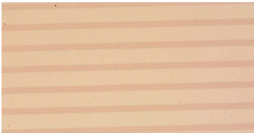
Figure 2.2. 10X bright field image of a HSC 11 OH stamped Au substrate after etching.
