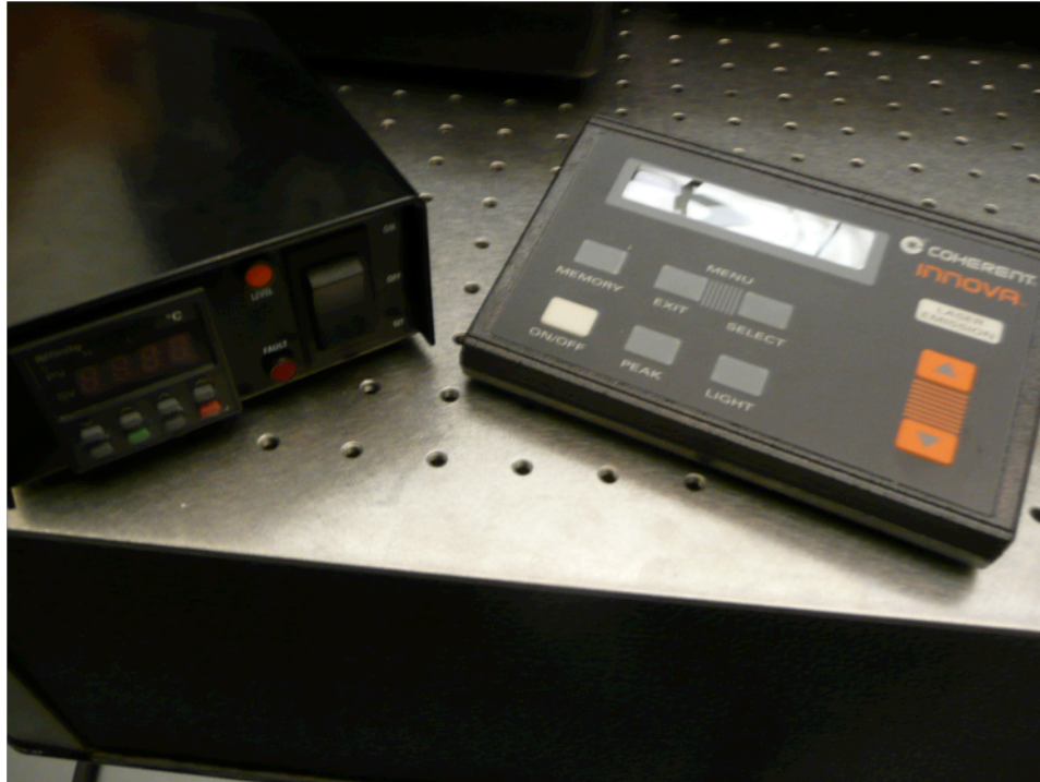
Figure A.2: The Affinity control module (left) used to change settings for the chiller and the Coherent control module (right) used to change the laser settings and read any error messages concerning the laser operation.
