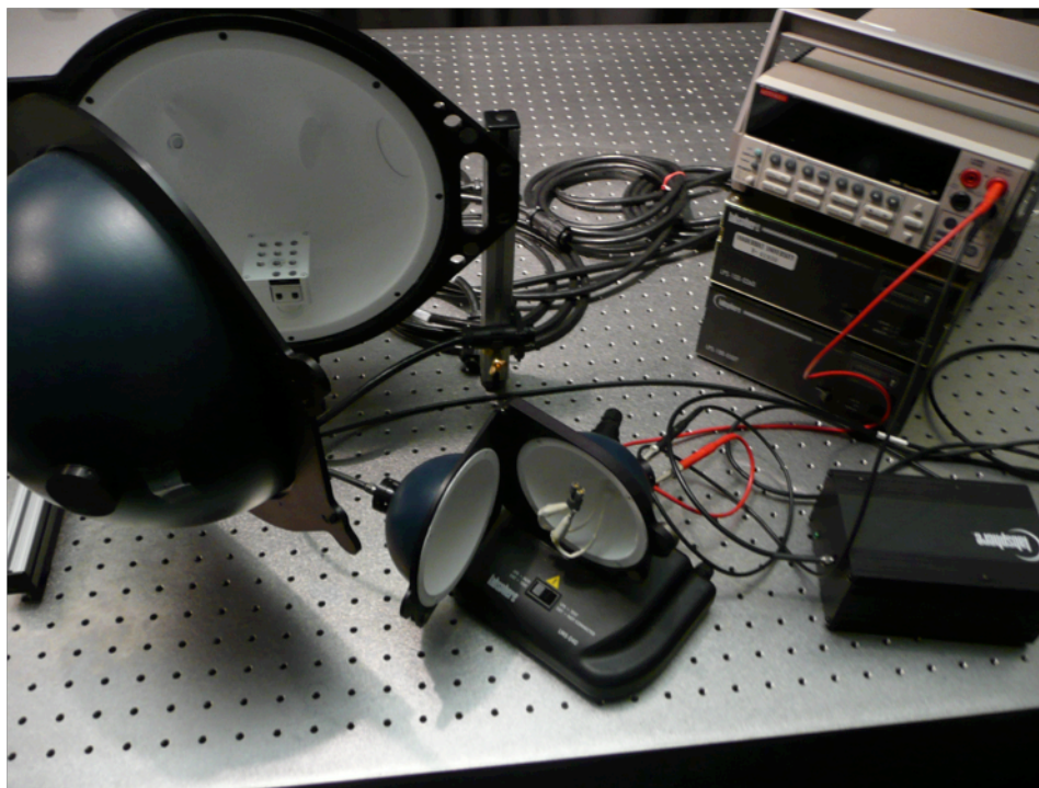
Figure B.1: The setup for measurement of LED sources and light emitted by nanocrystal-polymer films, including 4" (lower middle) and 10" (upper left) Labsphere integrating spheres, as well as the spectrometer module (lower right) and the power supplies that power the calibration lamps or LED sources (upper right).
