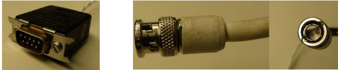
Figure 4. a) Preamp 9-pin male connector, b) Preamp BR2 male connector.
