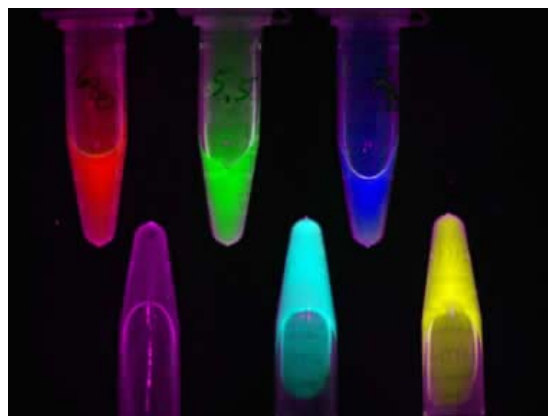
Figure 6.2. Spectral discrimination of five NIR dyes. The fluorescence spectra are color coded according to the spectrally resolved signal in the fluorescence image (one dye per tube; the 6 th tube = saline)
