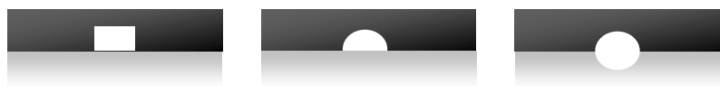
Figure 3.5. Three flow channel geometries: rectangular, semi-circular, and circular compared by ASAP during optical modeling of BI system.
