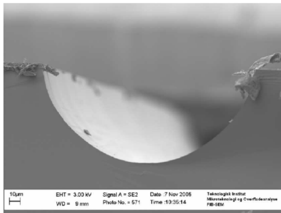
Figure 7.3. Semi-circular channel etched in Silicon with laser ablation being used to open the nitride mask for wet etching.
