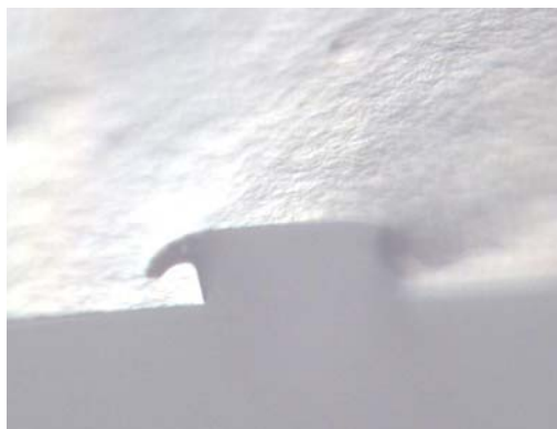
Figure 4.1. Example of T-topping from overexposure of SU-8 by low UV wavelengths.
