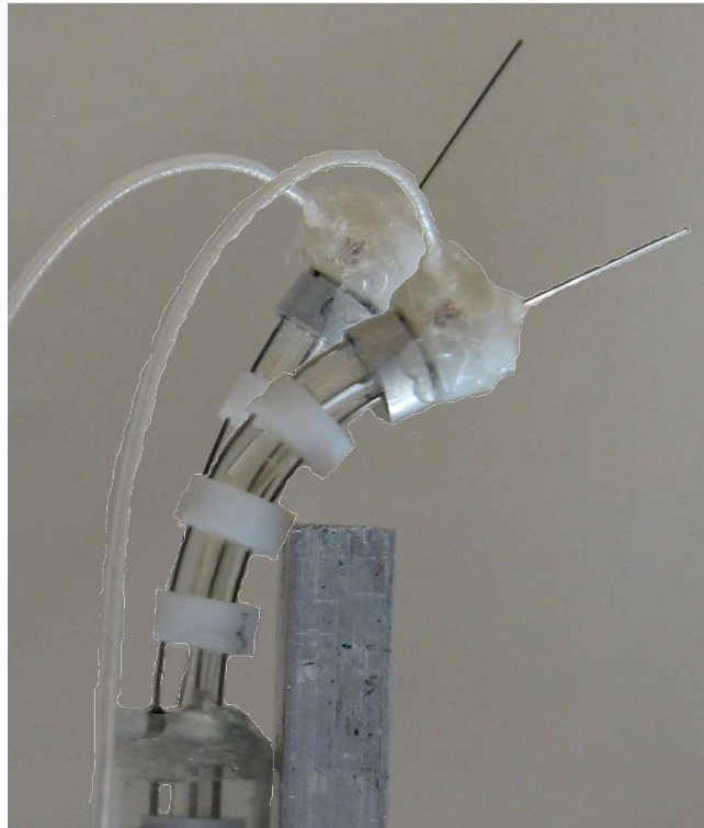
Figure II.3: Overlay of a single continuum segment before and after collision with a static object. The constrained part (bottom) remains fixed while the unconstrained part bends like a shorter continuum segment.
