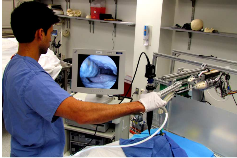
Figure VI.32: Experimental setup of the cadaveric evaluation of insertion and targeting of the voice box: 1) robots actuation unit, 2) cadavers head, 3) traksSTAR 2 flat transmitter, 4) bronchoscope, 5) visualization station, 6) surgeon.
