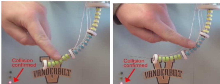
Figure IV.13: Effects on shape deviation when assumption A2 is violated.
