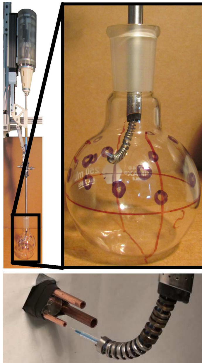
Figure VI.19: The experimental setup consists of a 7-axes actuation unit, a urologic resectoscope, a 2-segment continuum robot, a 250 ml beaker, and three tubes with various diameters. The beaker approximates the size of an average-sized bladder when inflated while the tubes were used for testing targeting accuracy.
