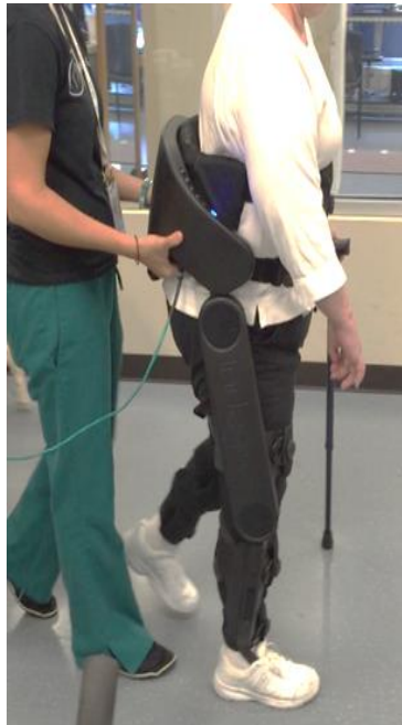
Figure 4.4. A subject walking in the Indego Exoskeleton. A PT is present to provide balance assistance if needed.
