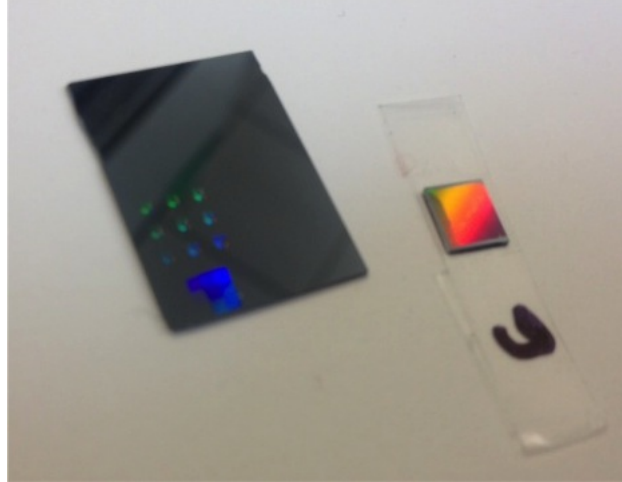
Figure A.2: Image of various stamp patterns on a source wafer and a stamp after being cut out and properly mounted on scotch tape.
