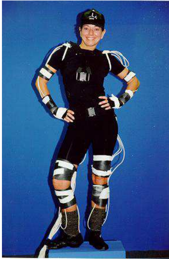
Figure II.3: A performer in a typical configuration of magnetic motion capture sensors. Image courtesy Bobby Bodenheimer.
