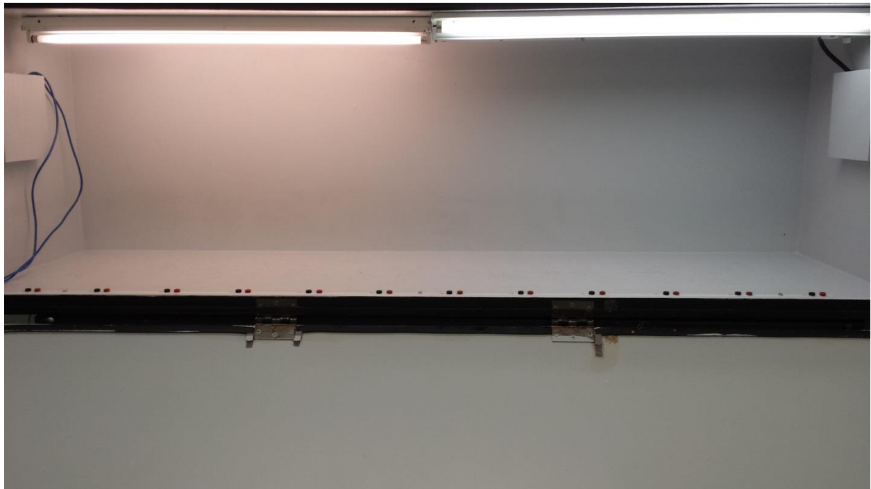
Figure A7. Light tight boxes in which animals were housed in order to control their light cycle. (A) Exterior. (B) Interior.
