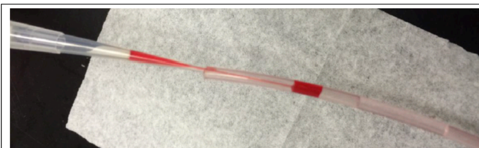
Figure 5. A gel loading pipette tip is also used to load the lysed blood and anit-PfHRP-2 magnetic bead sample into the tubing cassette.
