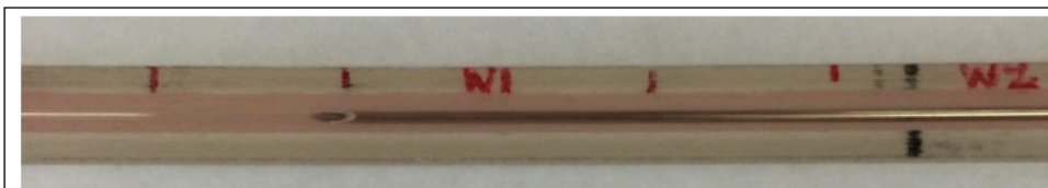
Figure 3. A 1mL syringe fitted with a needle is used to load wash buffers 1 and 2 into the proper locations in the tubing cassette.
