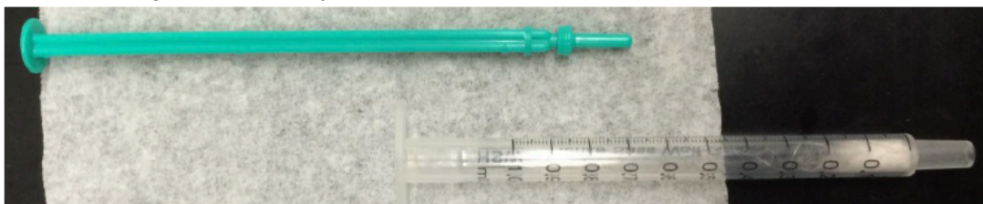
Figure 1. Lightly pack glass wool into a 1mL syringe to filter lysed whole blood samples before adding magnetic beads.
