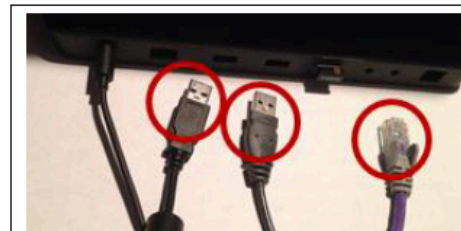
Figure 6. The connectors from the instrument to the back of the Surface Dock.
