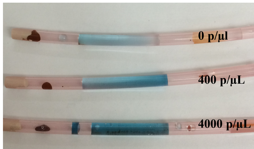
Supporting Information Figure IV. 5. Signal from 0, 400, and 4000 parasites/ \mu L after automated extraction.
