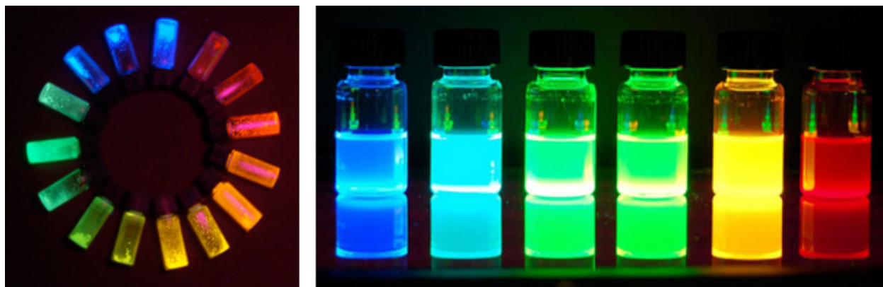
Figure 18. Examples of organic fluorophores (left) and quantum dots (right) in solution.
