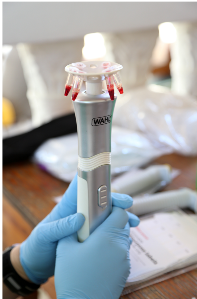
Figure 71. Lysed candidate patient blood samples processed using the handheld mixer designed by Dr. Nick Adams.
