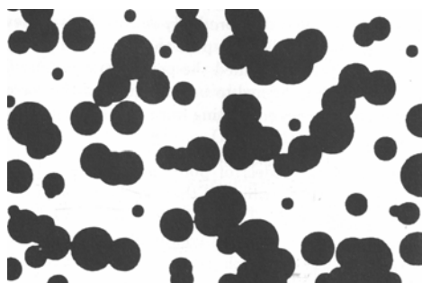
Figure 2-16. A Two-Dimensional Particle Packing Model of Randomly Distributed Disks (after Sahimi, 1995).
