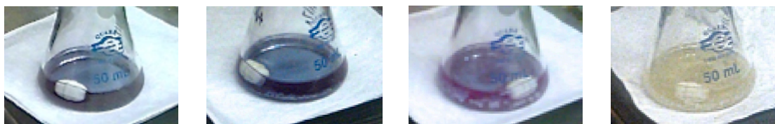
Figure 4. Reversible progression of \text{K}((3\text{-}t\text{-Bu})\text{tpy})\text{N}(\text{Si}(\text{CH}_3)_3)_2 solution from deep blue at room temperature (far left) to light yellow solution with white clusters at -35\text{ }^\circ\text{C} (far right).
