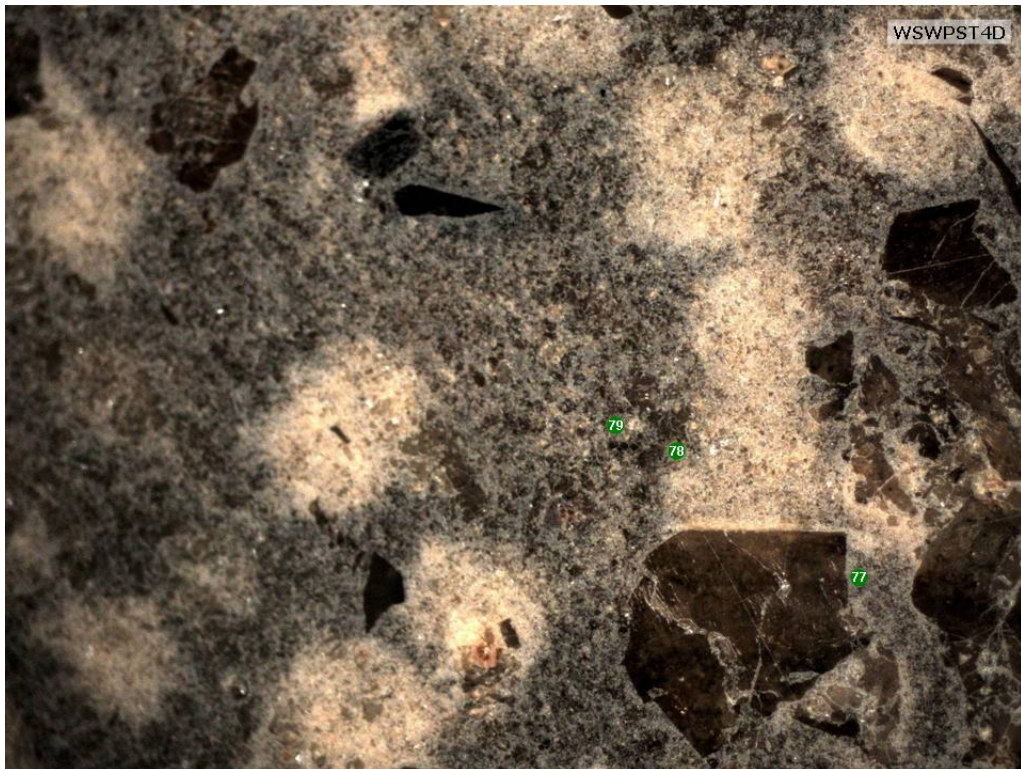
Figure B6. Photomicrograph of sample WSWPST4D with LA-ICPMS spot locations noted.
