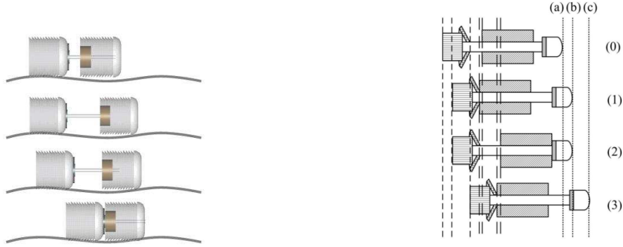
(a) Inchworm capsule by Kim et al. [73]. Impact-based piezo actuators and clamping devices create cycles of elongation, clamping and retraction.
