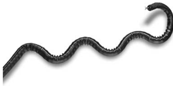
Figure 3.5: The continuum robot based endoscopic shaft of the Neoguide system. Reproduced with permission from [40] © 2006 Georg Thieme Verlag KG.
