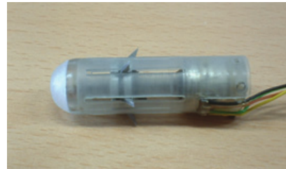
(b) Paddling capsule by Park et al. [106]. A linear actuator moves the legs up and down the length of the capsule much like paddles of a canoe.
