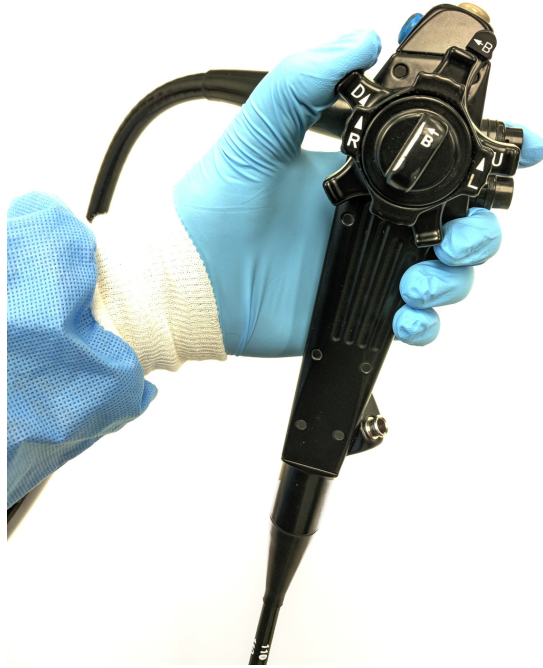
Figure 3.1: The user interface of the conventional endoscope. A physician controls the bending of the tip of the endoscope by rotating the control wheels at the base of the endoscope.
