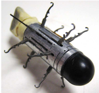
(a) 12 legged capsule by Valdastrri et al. [166]. The capsule had two sets of six legs that were controlled independently.
