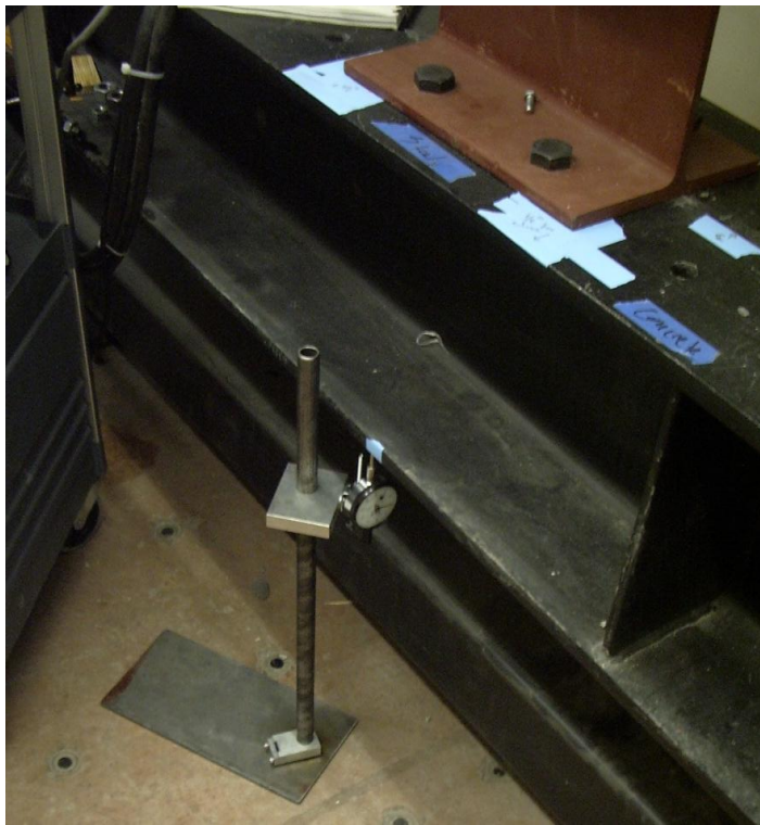
Figure 98. Dial gage under left test beam support
