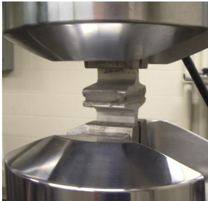
Figure B38. Sikadur 30 tensile specimen before loading
