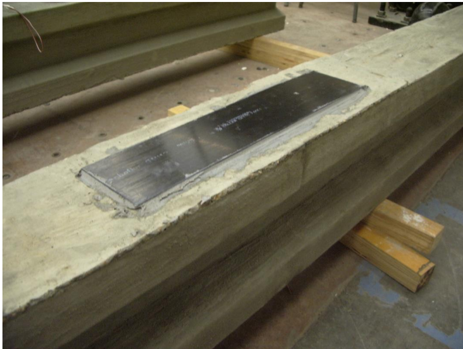
Figure 75. Completed Carbodur composite patch application
