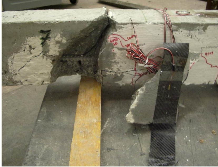
Figure 160. Final state of beam 7
