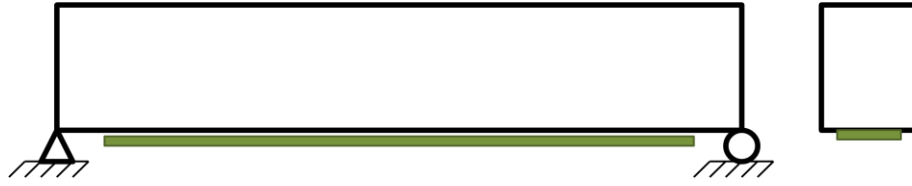
Figure 10. Common flexural reinforcing scheme
