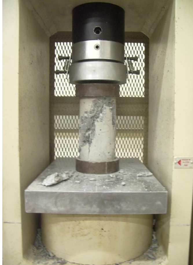
Figure 29. Typical test cylinder failure
