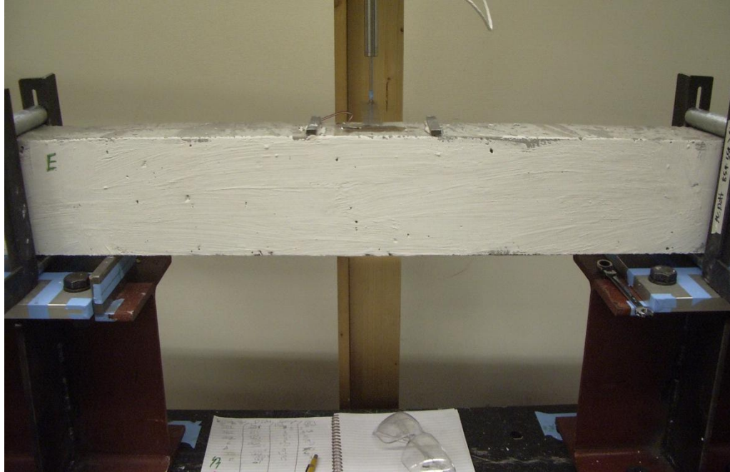
Figure 115. Typical concrete sample in loading devices
