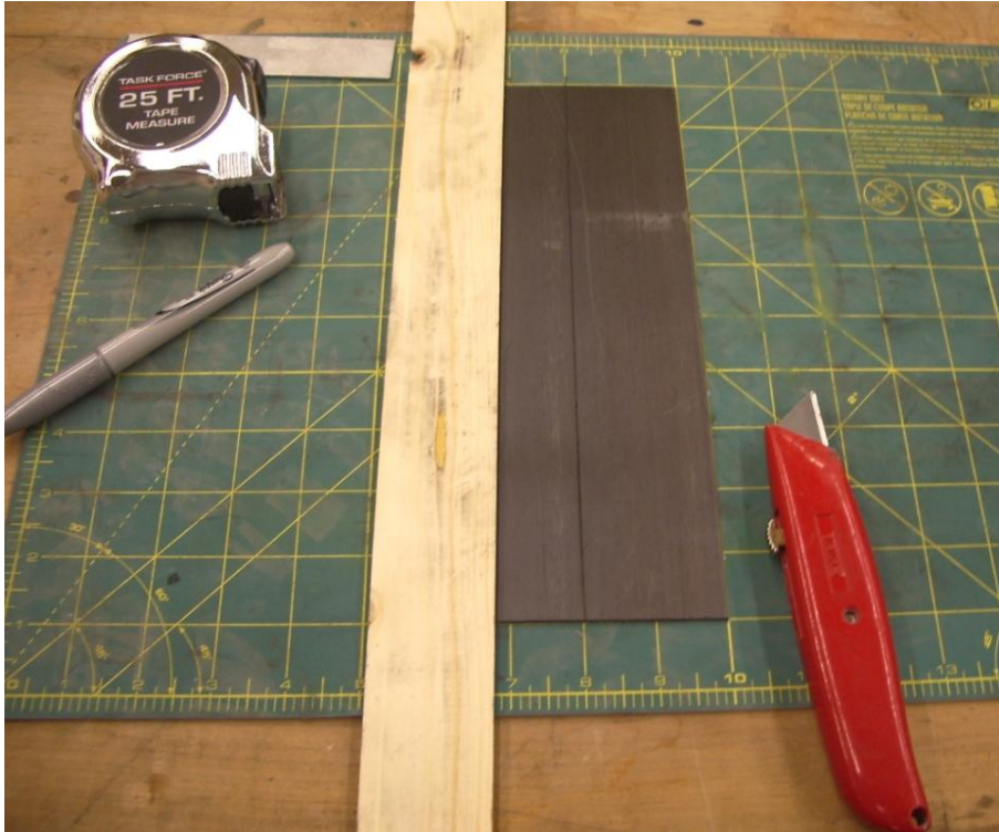
Figure 73. Typical cutting method for Carbodur patch
