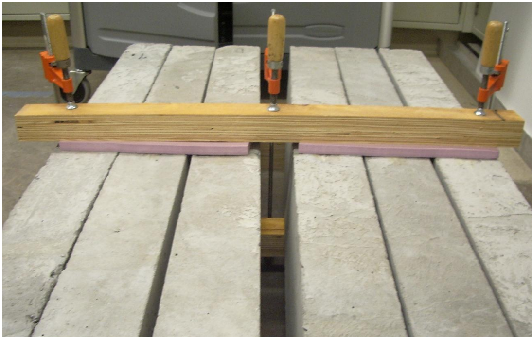
Figure 105. Concrete strain gages under pressure for proper epoxy adherence
