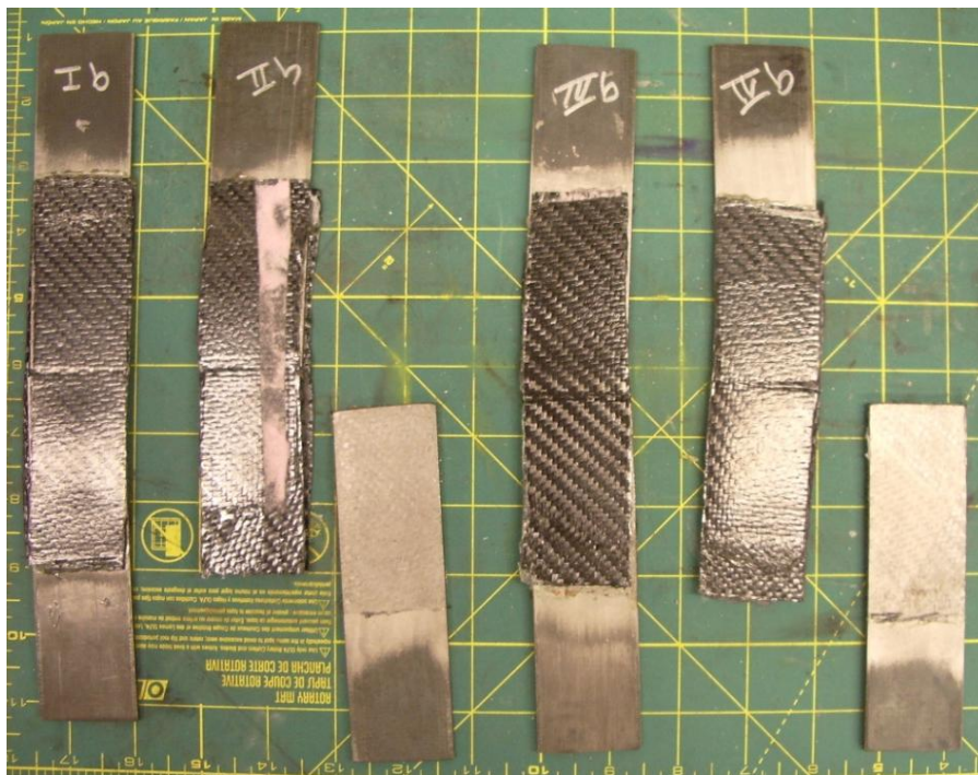
Figure B22. LTC 4300 shear specimens after failure, side a
