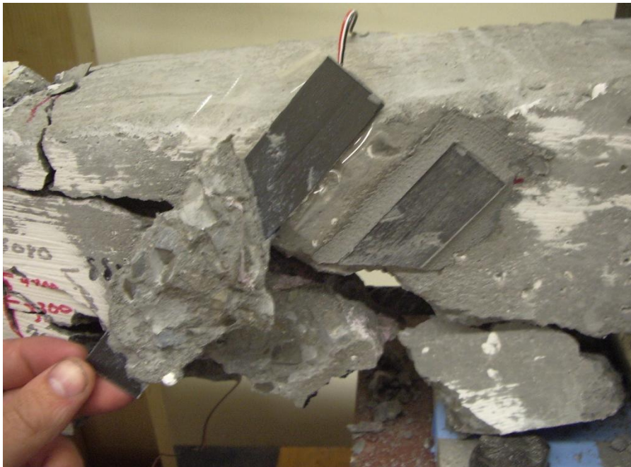
Figure 167. Concrete cover separation of test beam 9
