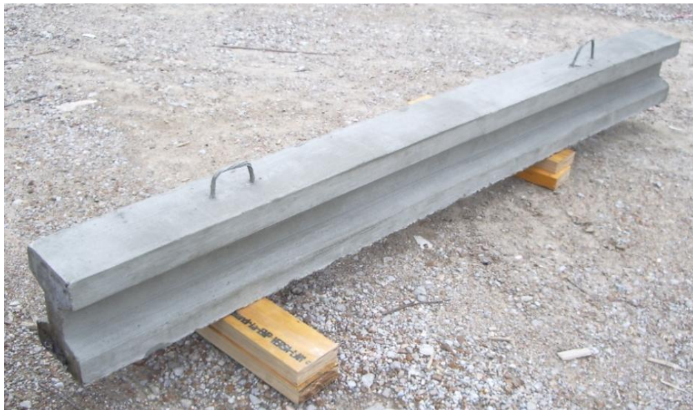
Figure 40. Prestressed beam before transportation to Vanderbilt laboratory facility
