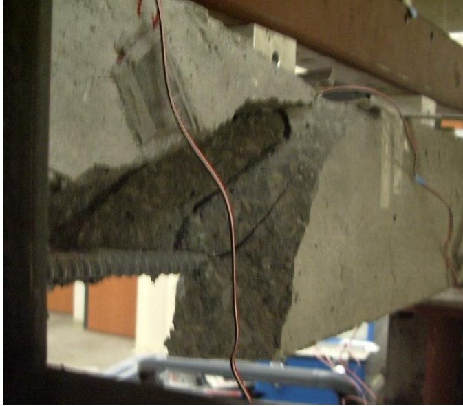
Figure 166. Far side of test beam 9 after failure
