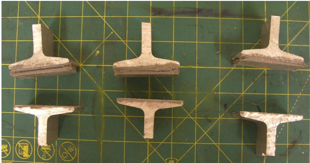
Figure B40. Profile of Sikadur 30 tensile specimens after failure
