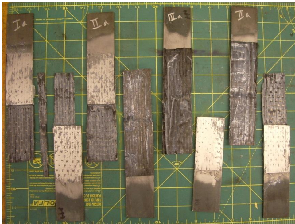
Figure B8. Sikadur 330 adhesive shear specimens, side a
