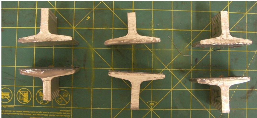
Figure B32. Side profile of Sikadur 330 tensile specimens after failure
