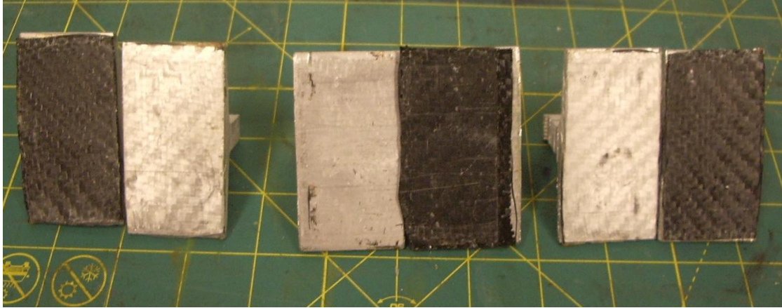
Figure B46. Surface of LTC 4300 tensile specimens after failure
