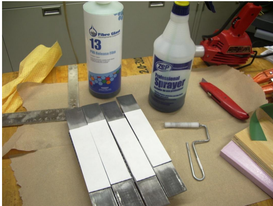
Figure 77. Components used to apply LTC 4300 composite to coupons
