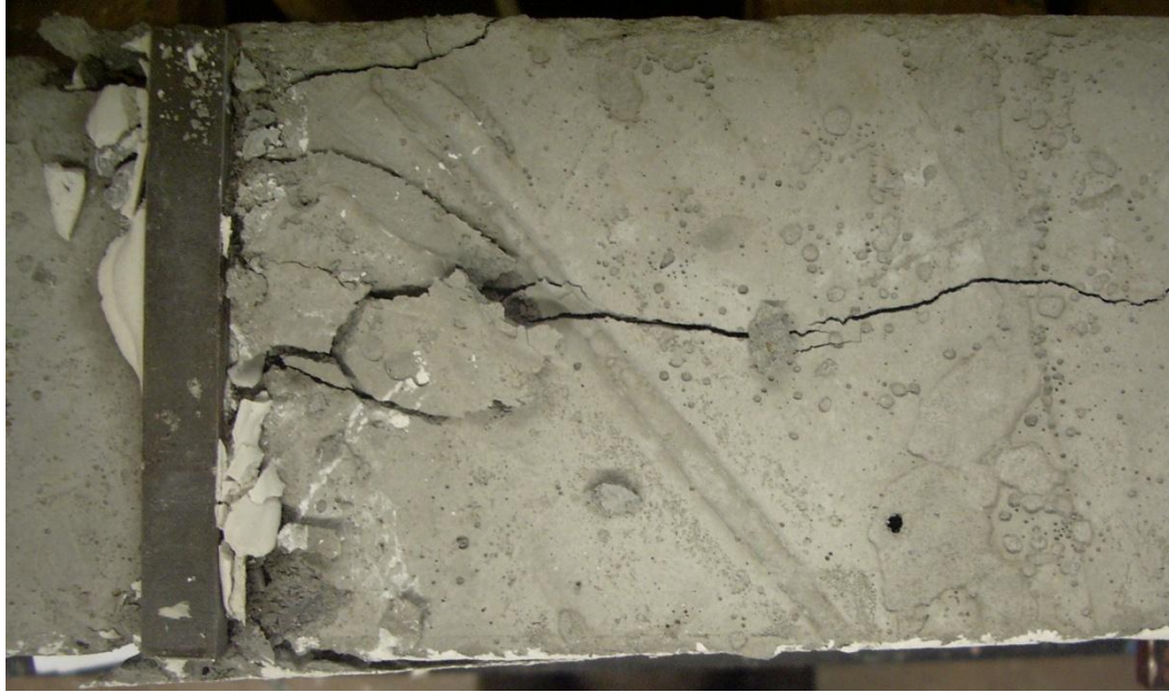
Figure 145. Top view of typical concrete crushing at point load application location
