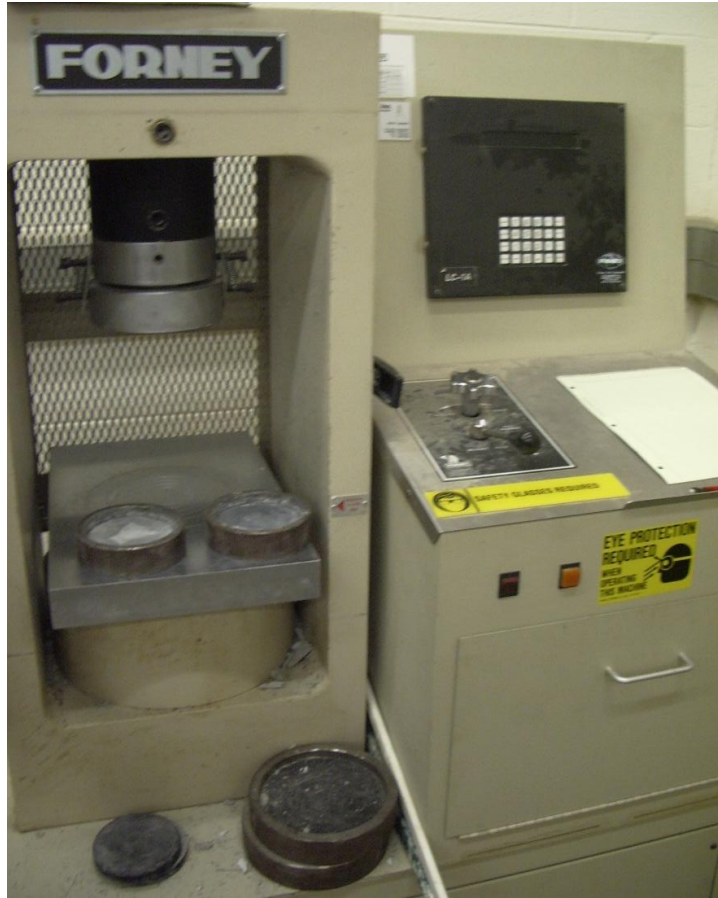
Figure 28. Machine for testing concrete cylinders
