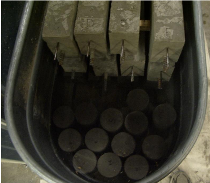
Figure 26. Concrete beams and cylinders being submerged in water
