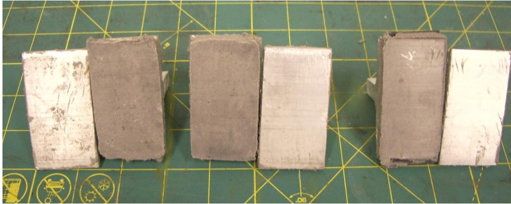
Figure B39. Surface of Sikadur 30 tensile specimens after failure
