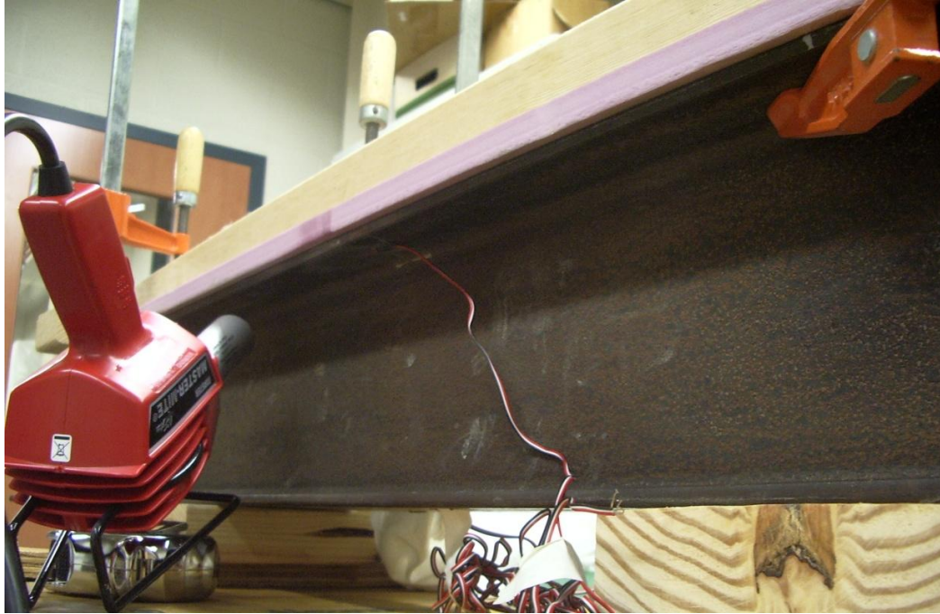
Figure 82. LTC 4300 cured to SBI with heat gun
