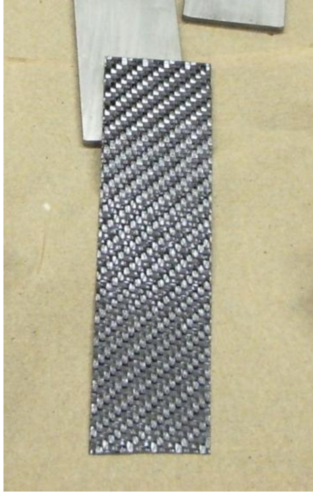
Figure 44. 6" x 1.5" sample of LTC 4200
