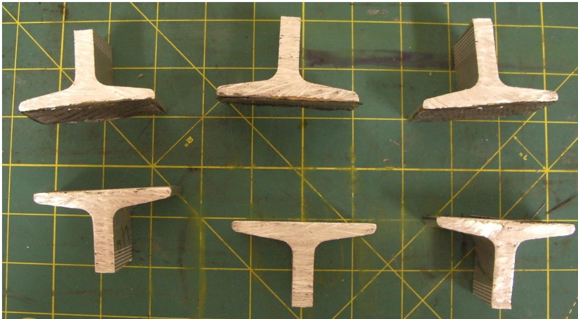
Figure B47. Profile of LTC 4300 tensile specimens after failure
