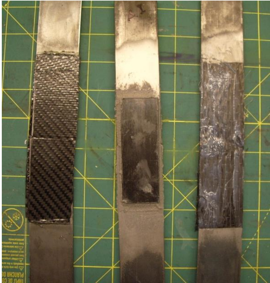
Figure B4. Finished LTC 4300 (left), Sikadur 30 (center), and Sikadur 330 (right) specimens
