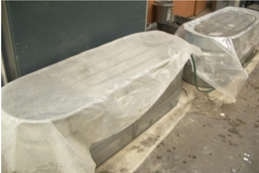
Figure 27. Covered tanks holding concrete beams and cylinders in water
