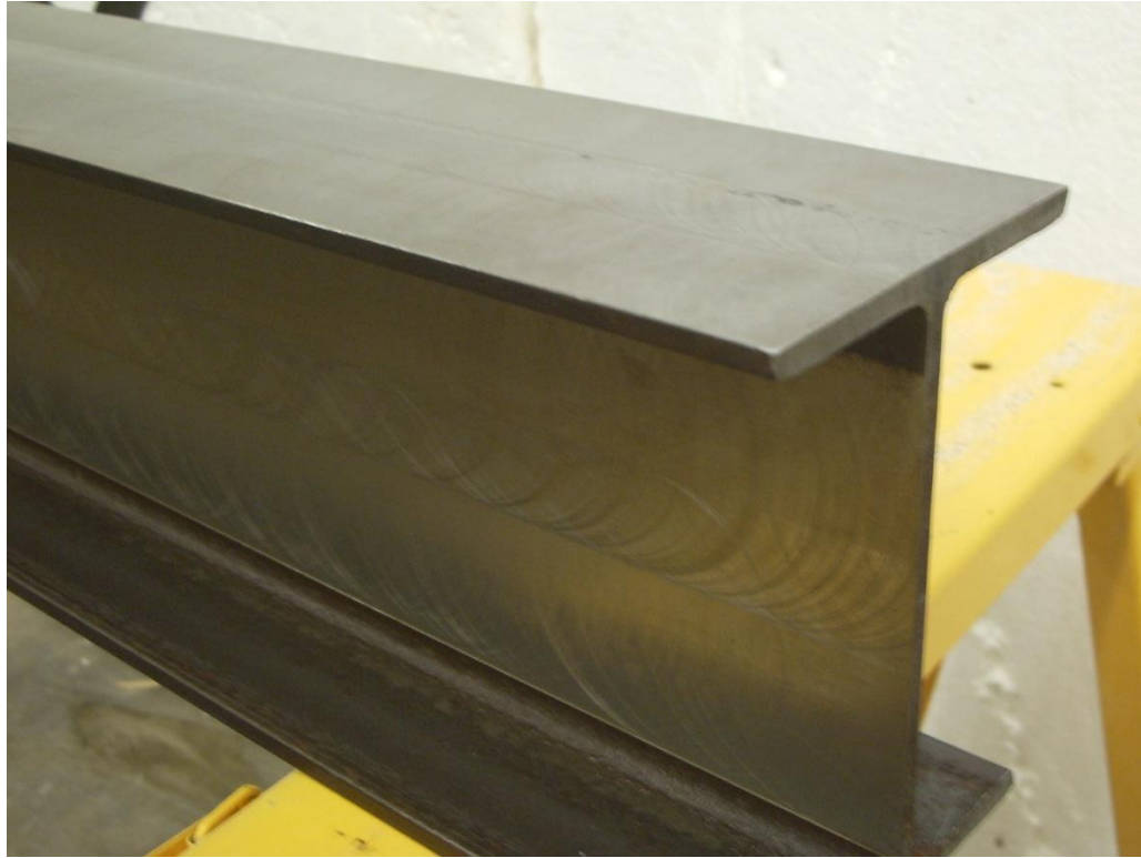
Figure 34. Milling marks show section loss of flange and web of beam SBIII
