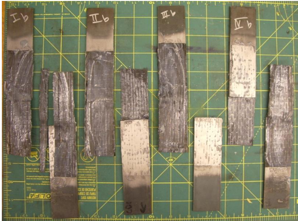
Figure B9. Sikadur 330 adhesive shear specimens, side b
