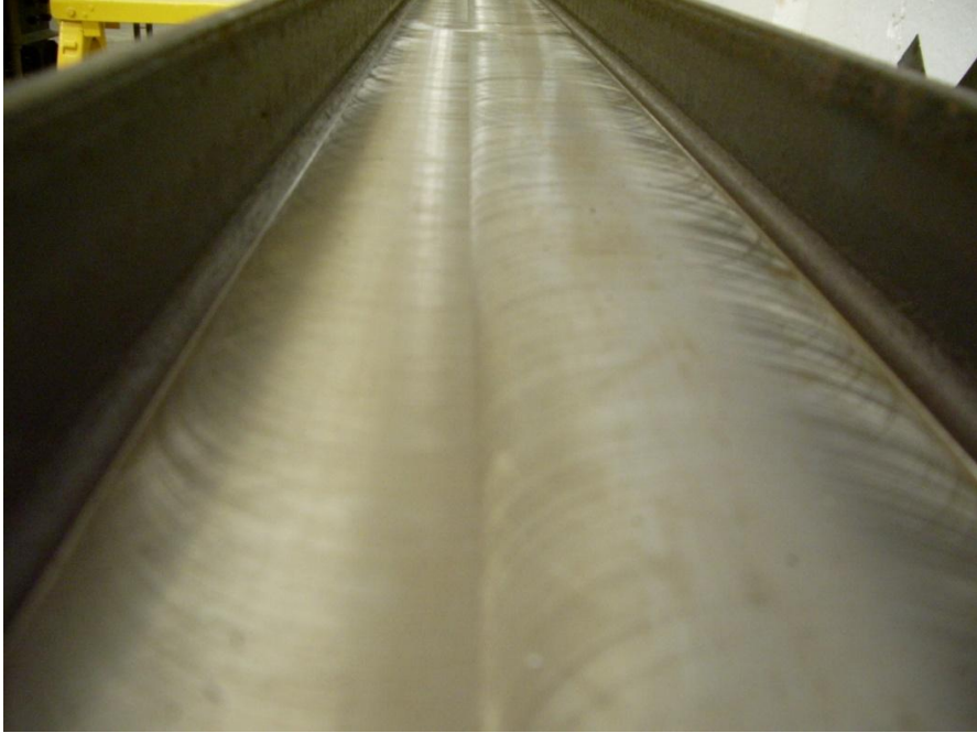
Figure 32. Close up view of milled web of beam SBII, side 1
