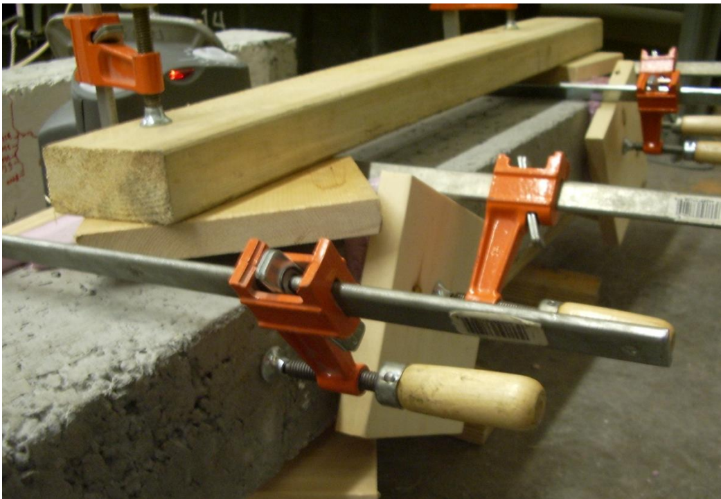
Figure 83. LTC 4300 cured to concrete beams with ceramic heater (background)
