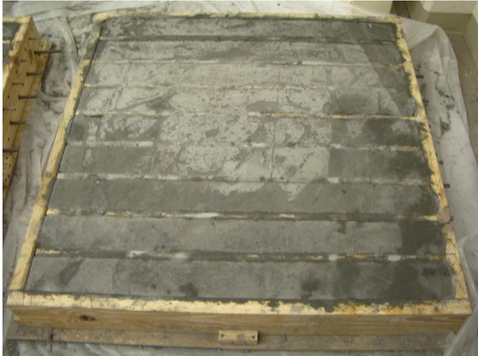
Figure 25. 3 flexural and 6 shear beams 24 hours after placement
