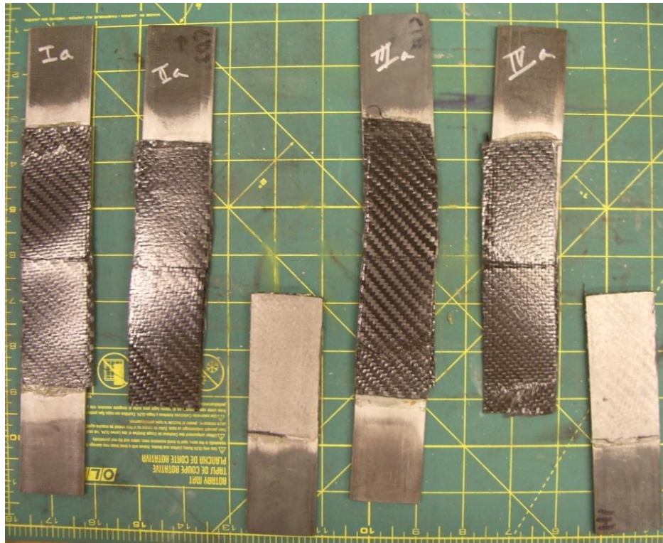
Figure B23. LTC 4300 shear specimen after failure, side b
