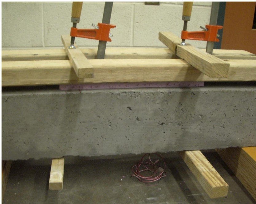
Figure 81. LTC 4300 clamped to reinforced concrete beams
