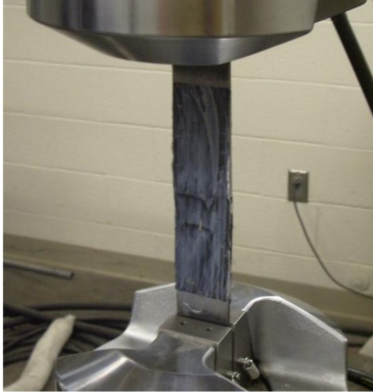
Figure B7. Sikadur 330/Sikawrap shear specimen before loading
