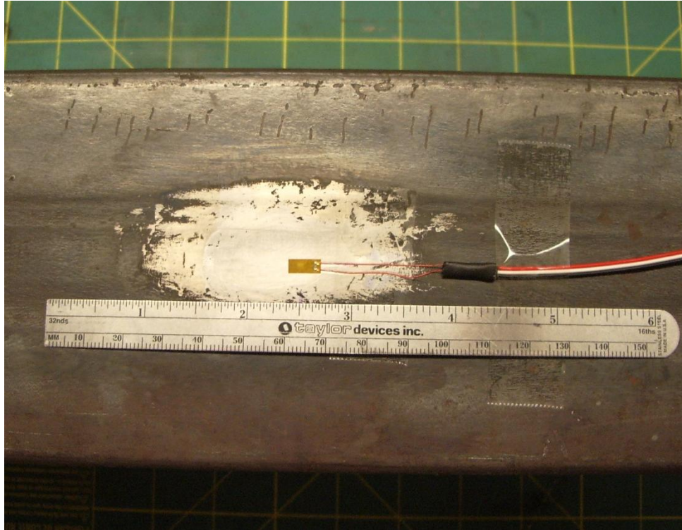
Figure 101. Typical strain gage instrumentation of top flange
