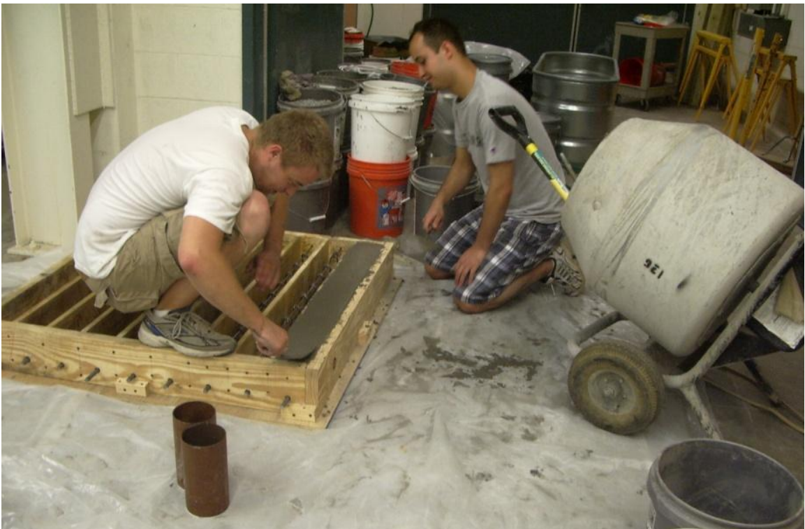
Figure 23. Reinforced concrete beams being placed
