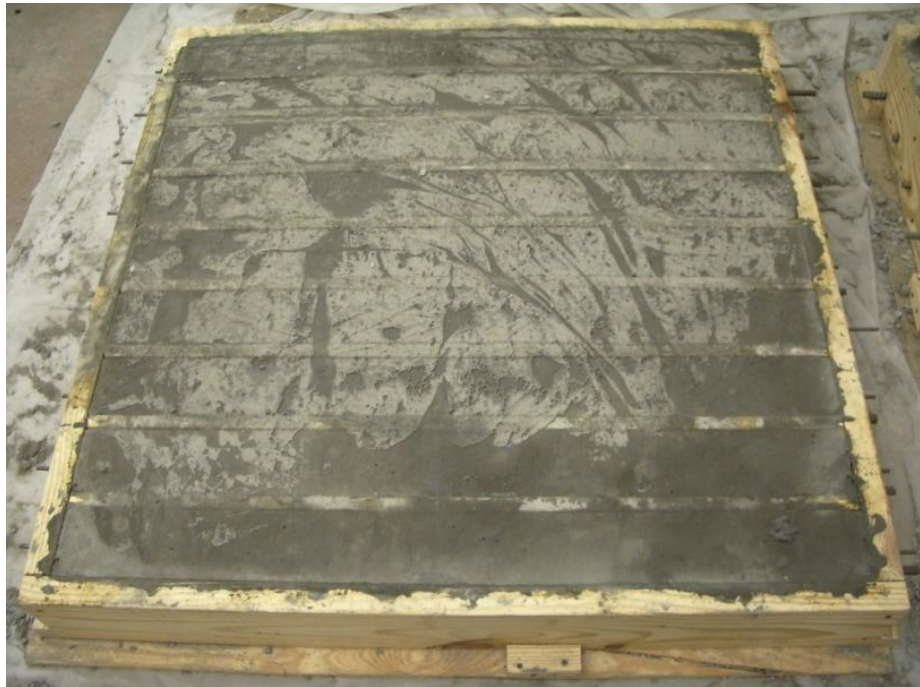
Figure 24. Flexural beams 24 hours after placement
