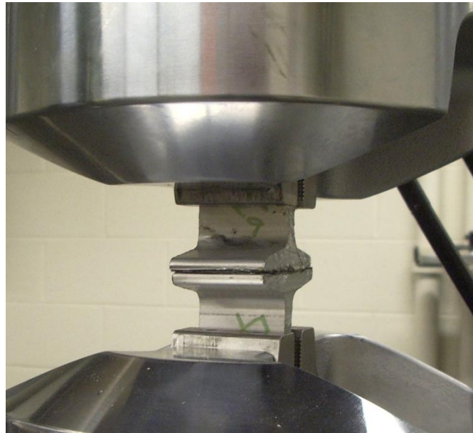
Figure B45. LTC 4300 adhesive tensile specimen before loading
