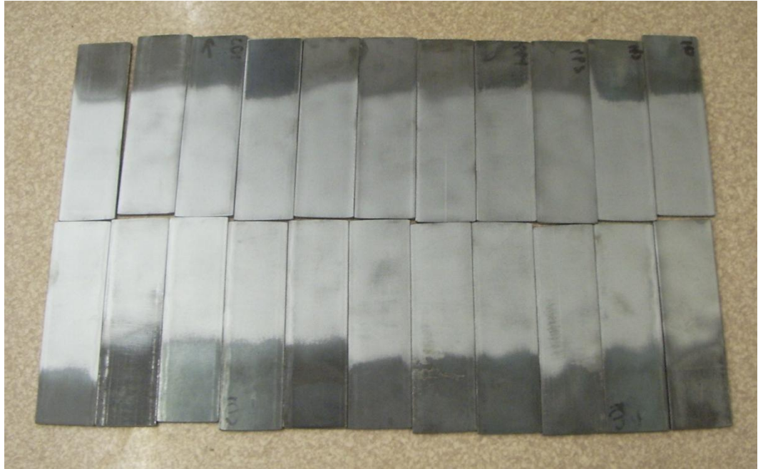
Figure B3. Plates for adhesive shear testing after bead blasting
