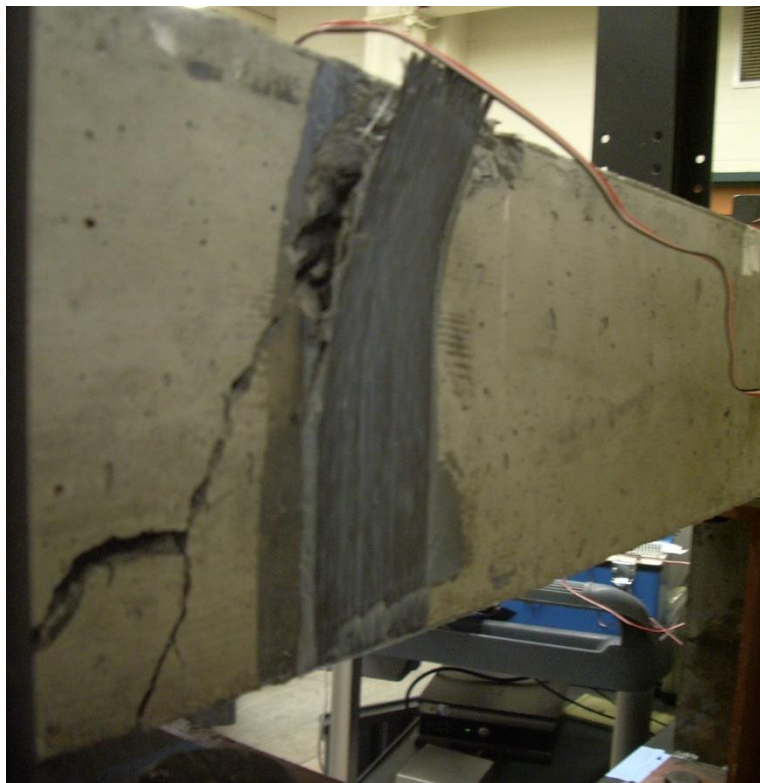
Figure 156. Concrete cover separation at patch location on the far side of beam 4
