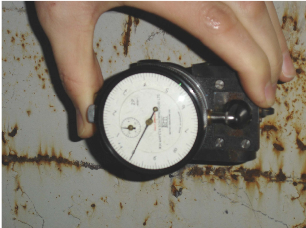
Figure 15: A closeup of the extensometer used to measure strain
