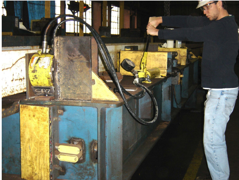
Figure 17: Load application using the hydraulic jack
