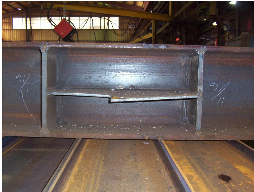
Figure 21: The buckled shear tab of test 1-1
