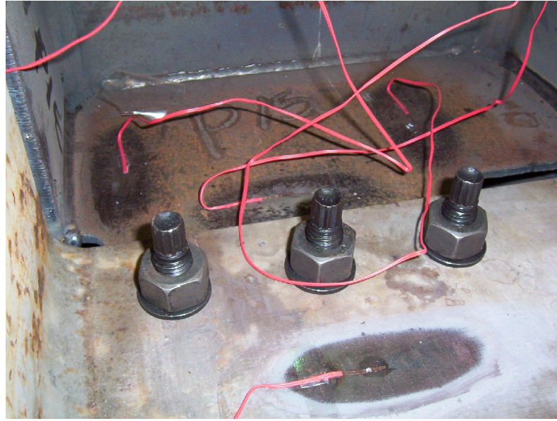
Figure 25: Strain gages at locations 2, 4, 5, and 6
