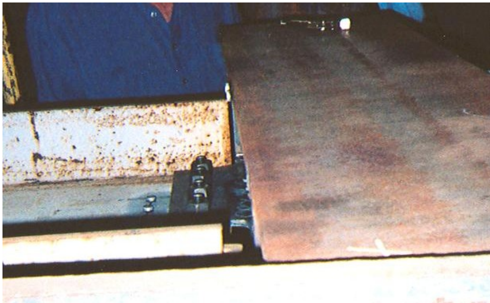
Figure 20: Rotation of the beam at the end of testing (space from flanges to column)
