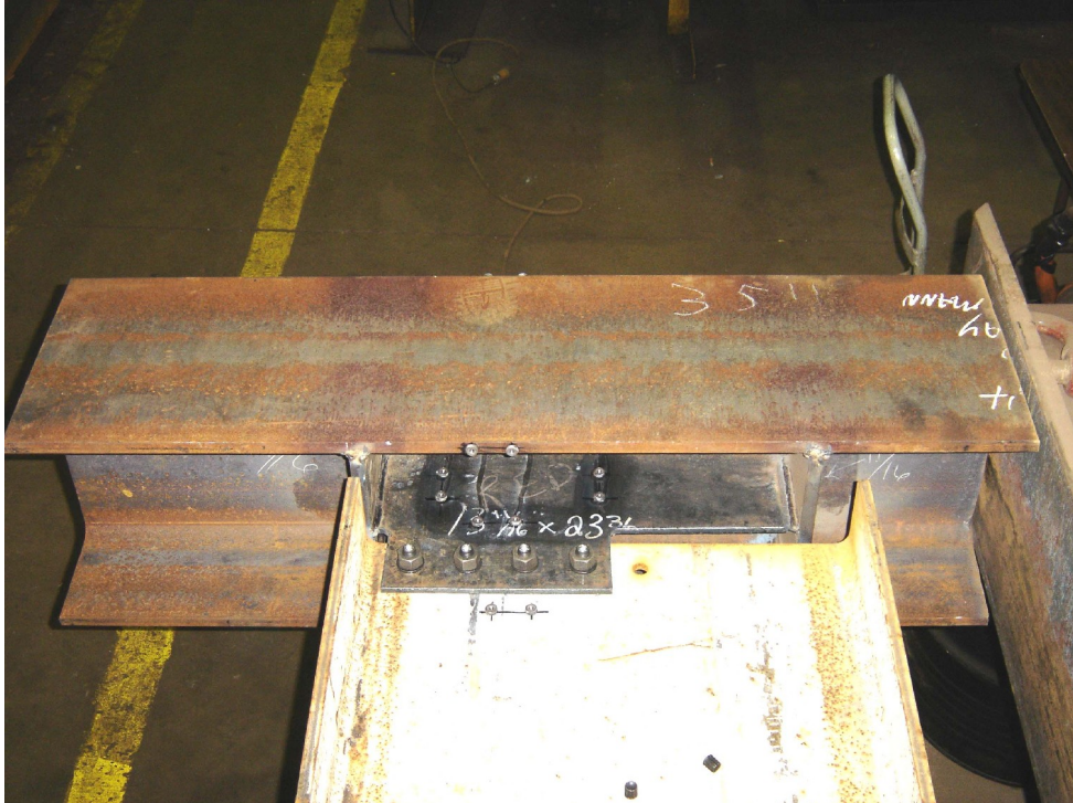
Figure 13: The connection, beam end and column stub before testing
