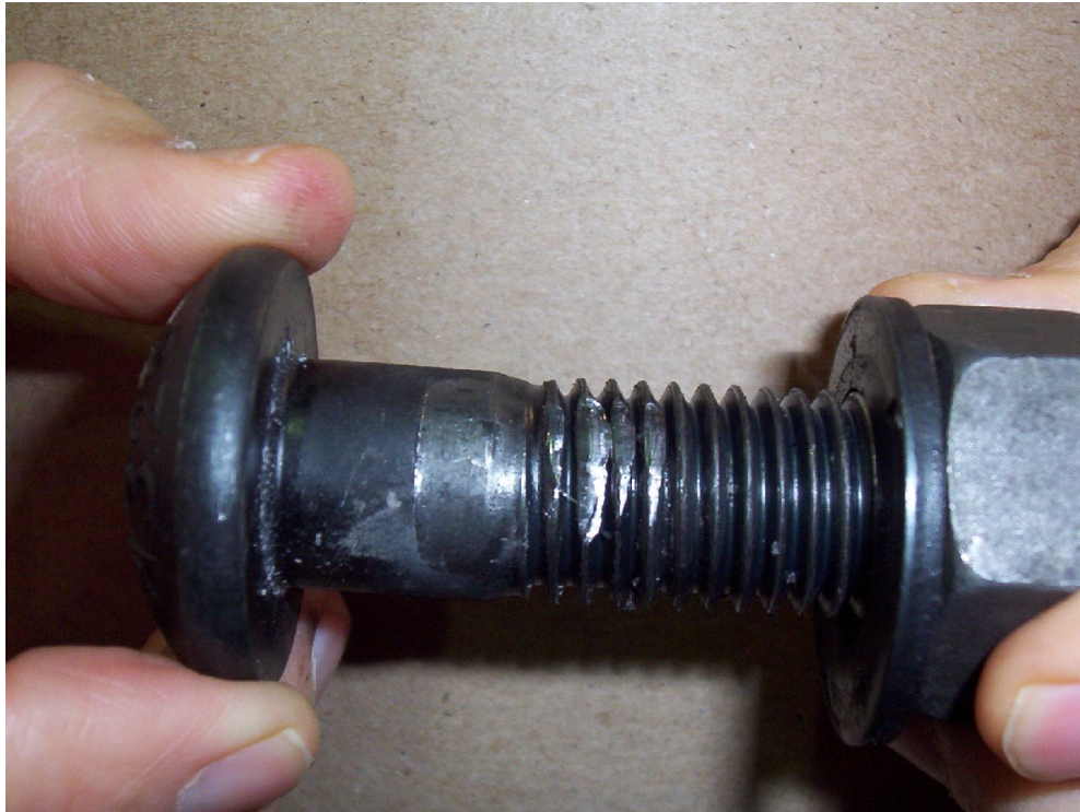
Figure 33: The deformation of the middle bolt from session 3 after the bolts were disconnected
