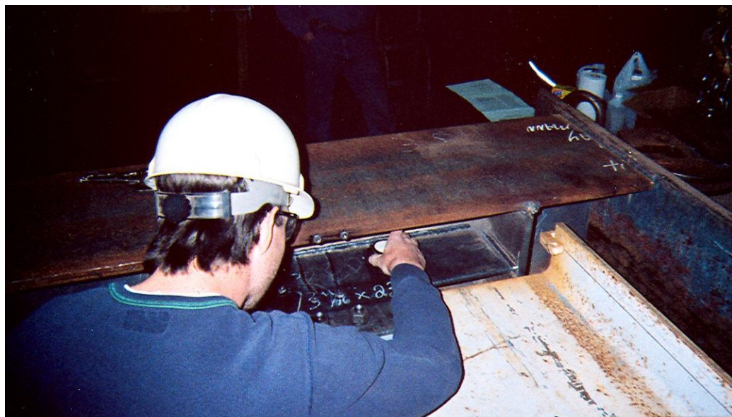
Figure 18: Using the extensometer to measure strain during testing
