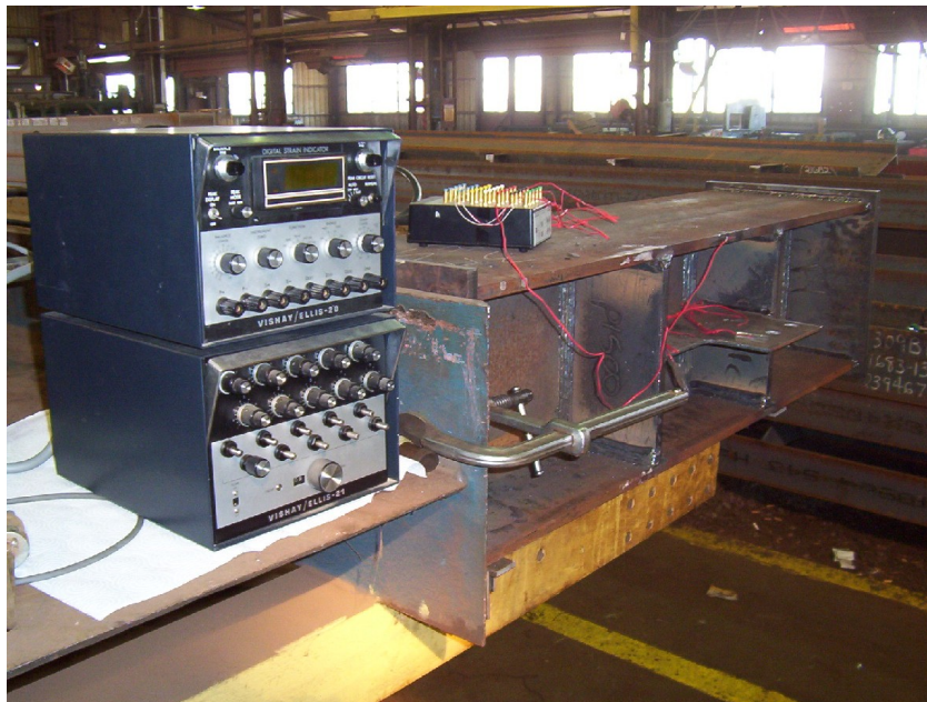
Figure 24: Equipment used to obtain readings from strain gages
