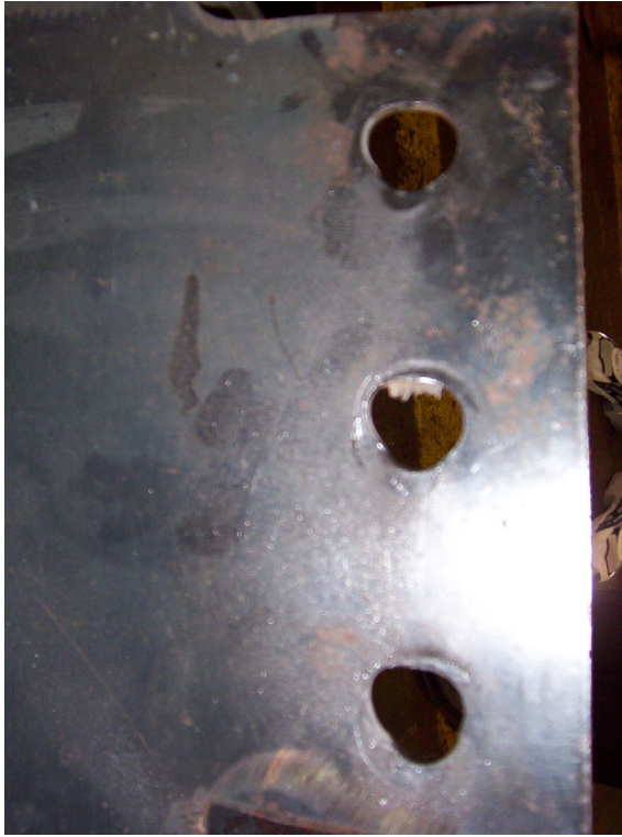
Figure 28: Deformed short-slotted holes after the test and disassembly
