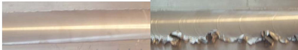
Figure 56 Comparison of favorable (left) and unfavorable (right) weld surfaces. Left image corresponds to 1000 rpm/5 ipm; the right image is the 1000 rpm/7ipm case.
