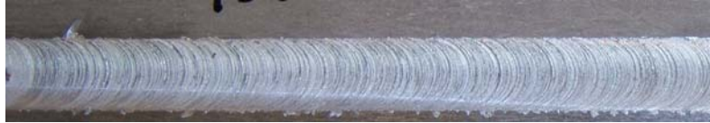
Figure 67 Welded surface of Al 6061/SiC/17.5p. Performed at 1250 rpm, 3 ipm using Trivex tool with self-optimized shape.
