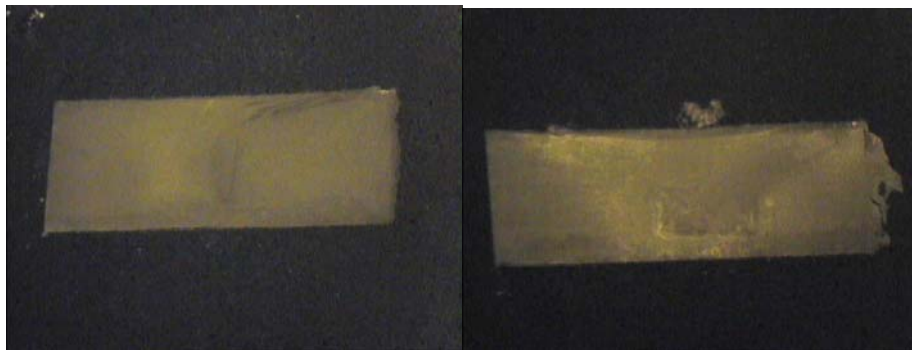
Figure 68 Sample macrographs for “good” welds at parameters in weld envelope. Corresponding parameters are 1250 rpm, 3 ipm (left) and 1000 rpm, 3 ipm (right).
