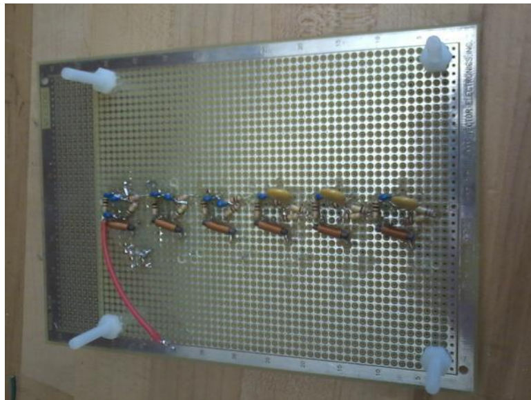
Figure 54. Next L1, the inductor, was put in place
