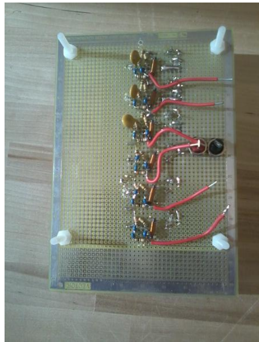
Figure 56. The remaining components for each circuit were put in place and the banana jacks were added. Then the circuits were tested to ensure that having multiple converters on one power line would not cause inappropriate operation
