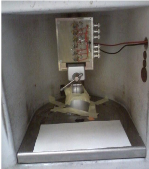
Figure 18. Irradiation setup in the Shepard Cell Irradiator
