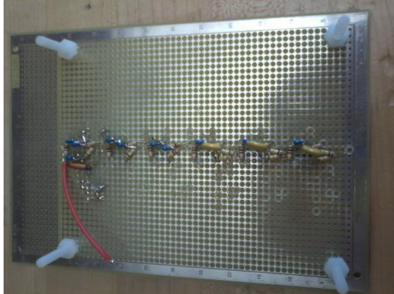
Figure 53. Next R1 and C2, the compensation resistor and capacitor, were put in place
