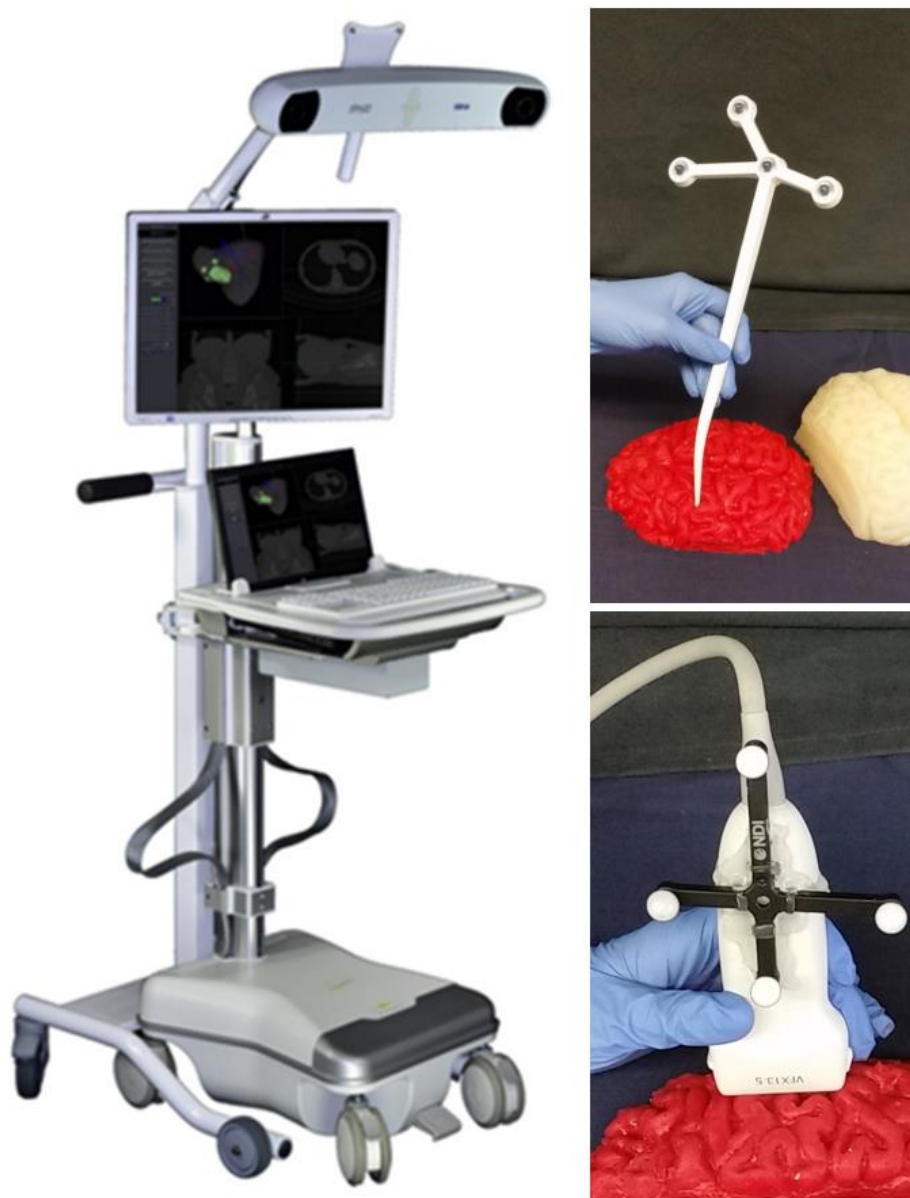
Figure III.1. Example setup of image-guidance hardware. (Left) A Polaris Spectra camera system and OR cart. (Right, top) A passively tracked manual-stylus used for surface data collection and organ interrogation. (Right, bottom) A passively tracked ultrasound probe.
