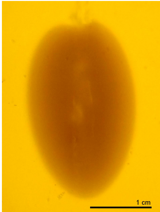
Fig. VI.2. Sample backlit mock histology of ablation zone (cut along the axis of the Perseon ST antenna) following an ablation at 60 W for 15 minutes in an agar-albumin phantom.
