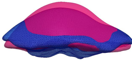
Fig. IV.2. The CT segmented preoperative and intraoperative phantom surfaces are presented in red and blue respectively. The differences in surfaces highlights the volumetric deformation undergone in the simulated phantom data. (© 2017 IEEE)
