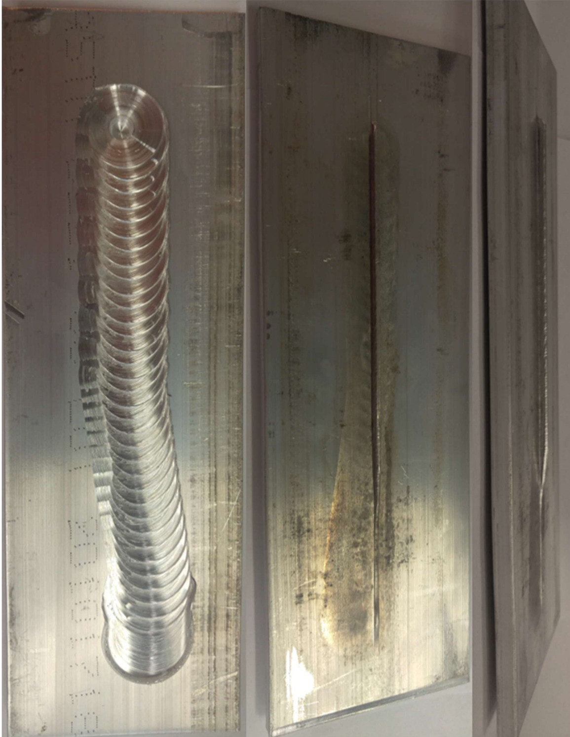
Figure 45: Top, bottom, and side view of weld 3
