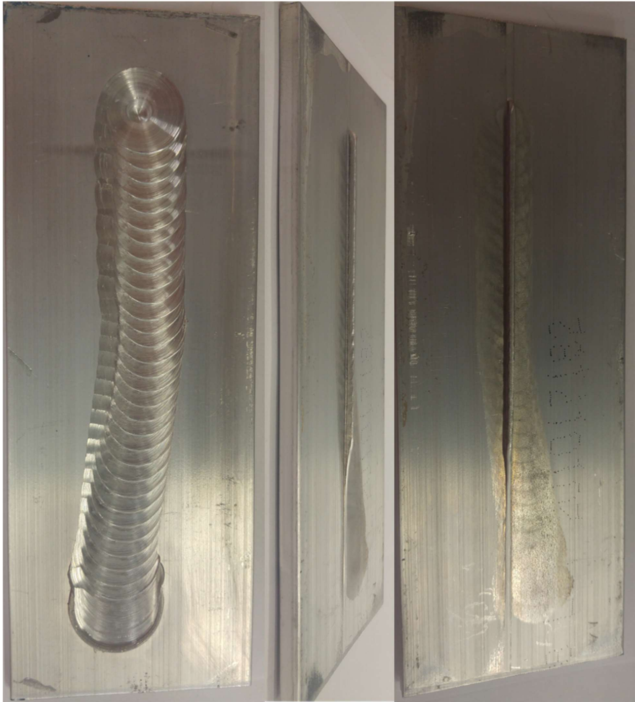
Figure 46: Top Bottom and Side view of Weld 2
