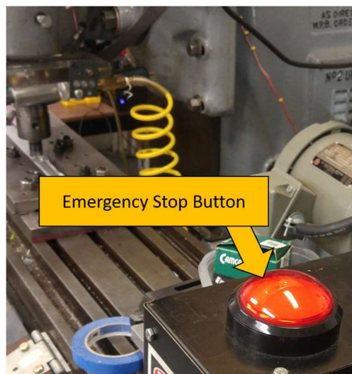
Figure 11: Emergency Stop Button
