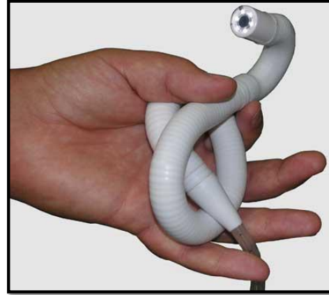
(b) Endotics teleoperated flexible endoscope [16]
