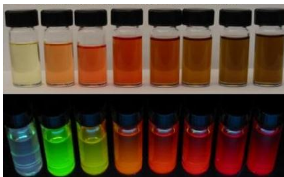
Figure 1.2: CdSe nanocrystals with diameters 1.7-5.2nm, arranged by size with the smallest on the left. The NCs above are under normal room light. The same NCs below are under UV light. 11
