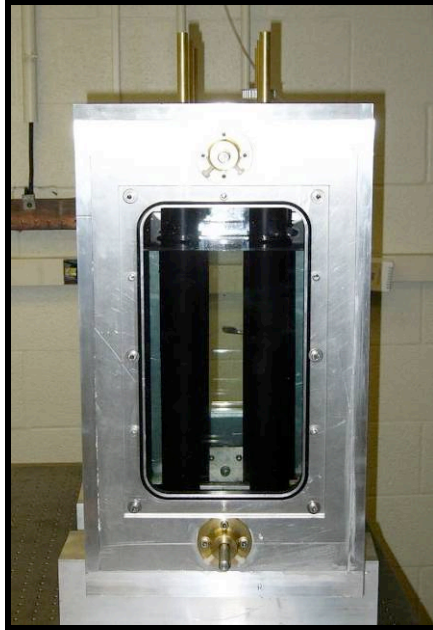
Figure 7. Side view of cavity system looking parallel to the internal moving boundaries as viewed by the observer.
