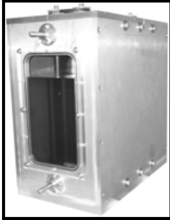
Figure 5. Side view of glycerin filled tank showing the structure, acrylic sidewalls, and adjustable sidewalls.
