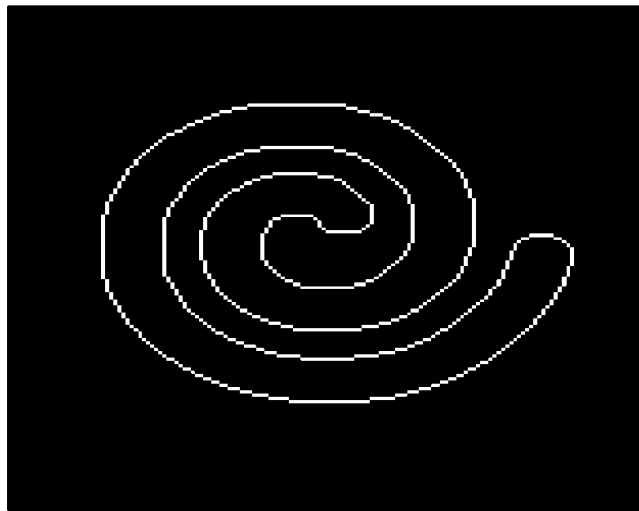
Figure 4.2: Image of the edges of the same nanospiral as in figure 4.2 using the Matlab® defined edge function. The white line represents the edge of the nanospiral.
