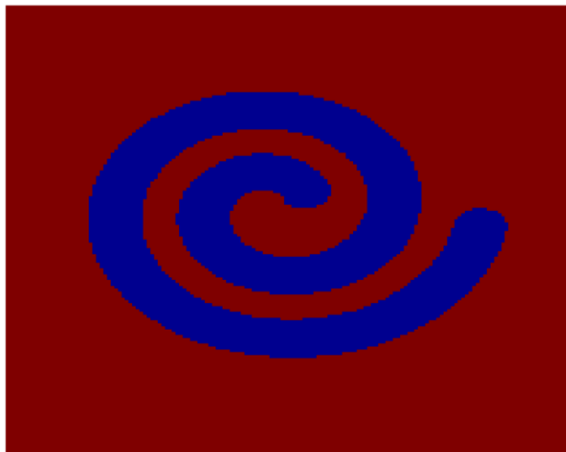
Figure 4.1: Image of the index of refraction for a simulated 60nm spaced, 40nm width nanospiral. The red region is void and the blue region is Au.
