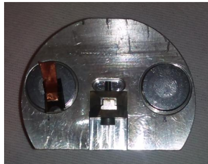
Figure 2.4 The “TEM” holder for FIB lift-outs on the Zeiss Auriga. To the left and right are sample holders, while the center is reserved for a lift-out grid (sandwiched between two metal plates).
