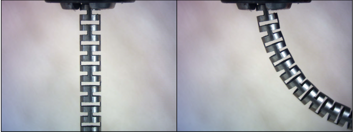
Figure 4.9: Magnified views of the transition section of the dexterous sheath. This section is designed to be highly flexible to pass through the S-curve of the setup sheath.
