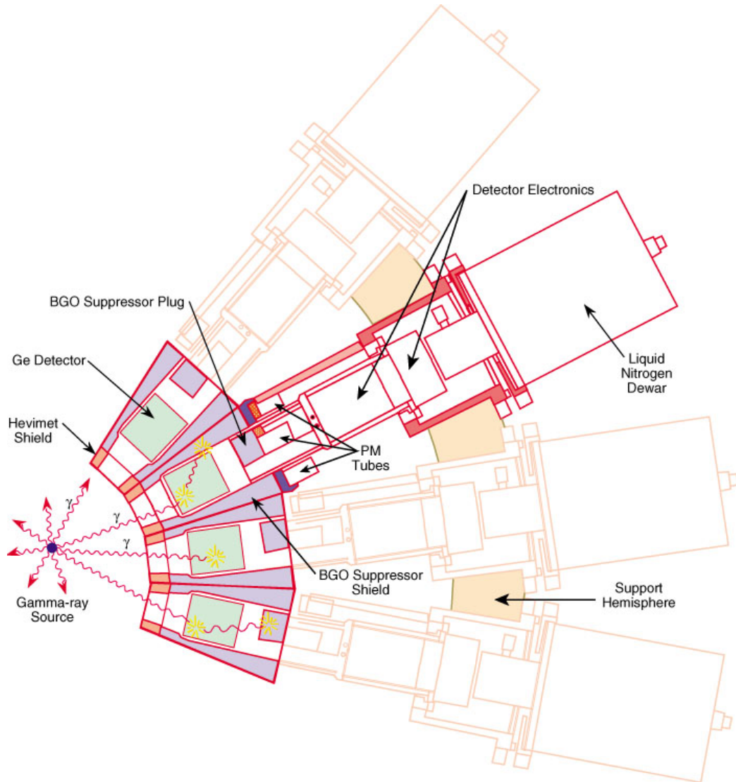
Figure 4.3: A cross section schematic of Gammasphere [43]
