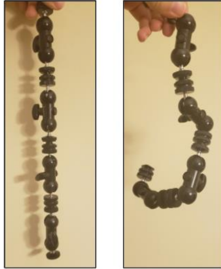
Figure 11. Prototype v0 in flexible (left) and rigid (right) states.
