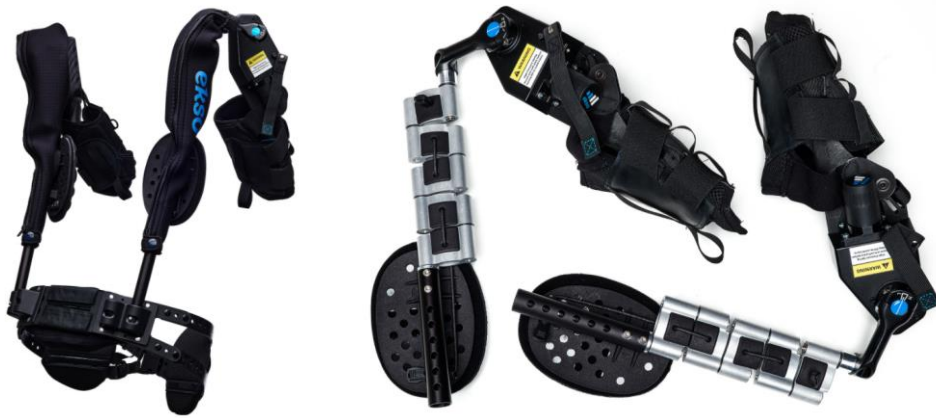
Figure 1. EksoEVO wearable exoskeleton [2].
