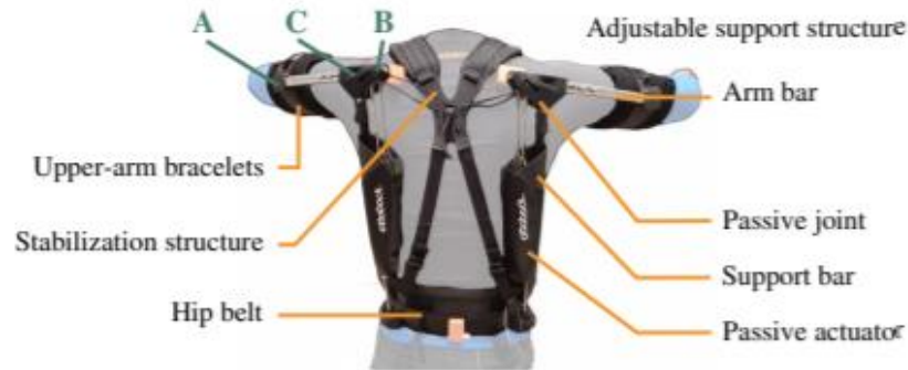
Figure 3. PAEXO Shoulder wearable exoskeleton [9].
