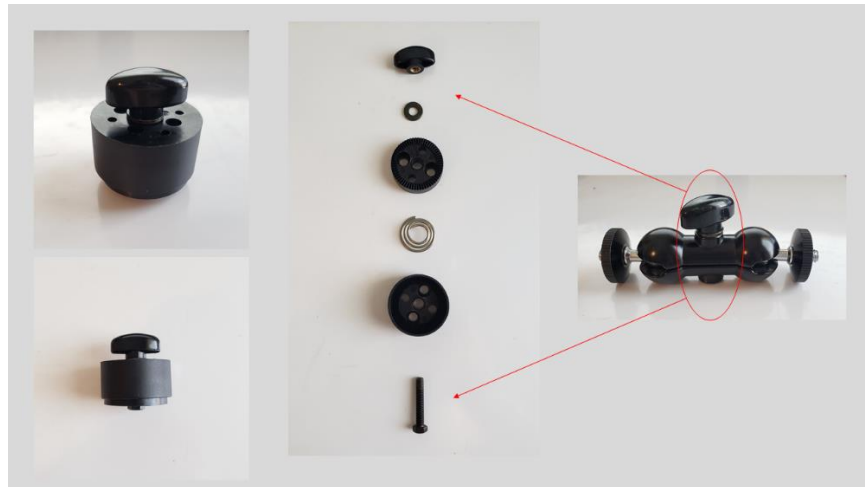
Figure 16. Prototype v2 locking mechanism proof of concept.
