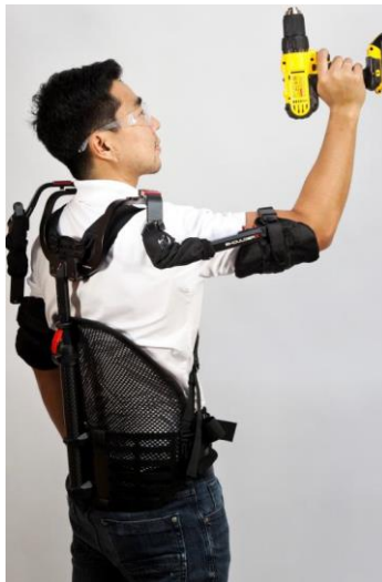
Figure 2. SuitX's shoulderX wearable exoskeleton [5].
