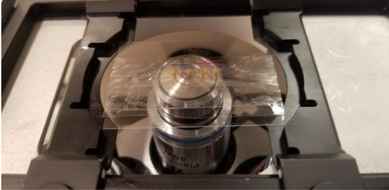
2. Move the stage to aim the laser to the desired region of the pupa. In this case, the laser ablates at the center of the frame, so the stage is aligned accordingly.
