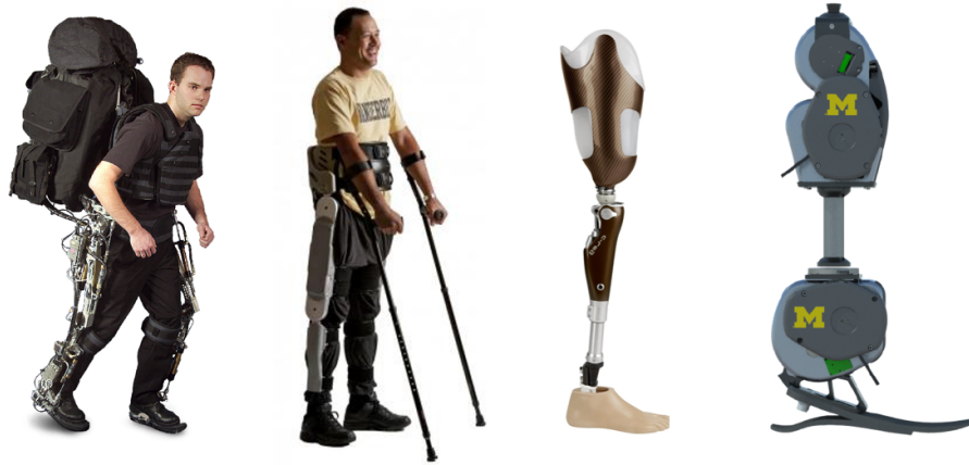
Figure 1.1: Examples of lower-limb wearable assistive devices. From left to right, Berkeley Lower Extremity Exoskeleton (BLEEX) [128], Parker Indego, Ottobock C-Leg, Michigan Open-Source Robotic Leg [3]
