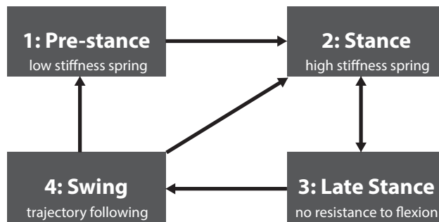
Figure 6.2: Finite-state machine for powered knee prosthesis closed-loop walking controller.
