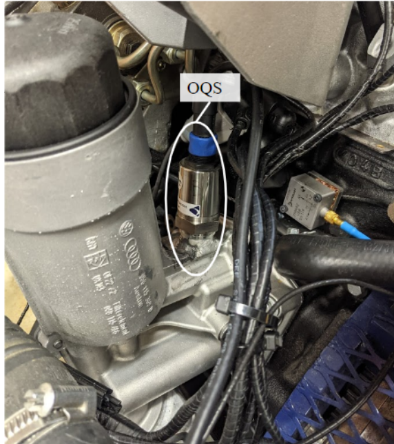
Figure 4.1: Vertical OQS as installed at the oil filter housing on the engine. Oil temperature was monitored by the built-in thermistor on the OQS (Figure 3.1).
