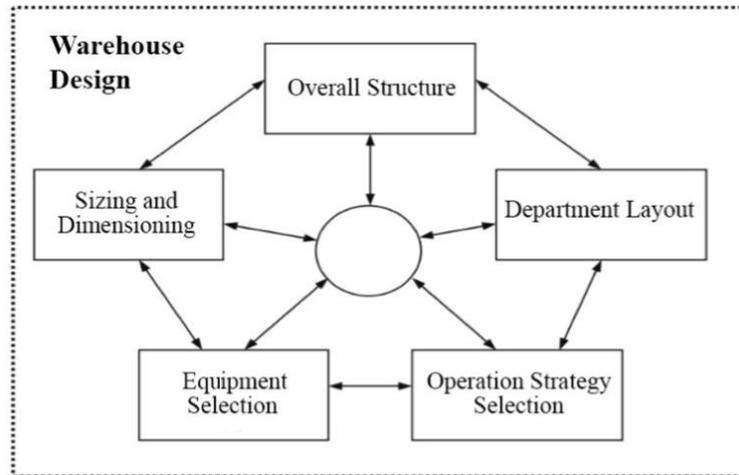
**Figure 2: Foundational elements of warehouse design**
