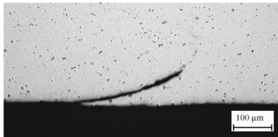
Figure 10: A weld line flaw from [Threadgill, 2007]
