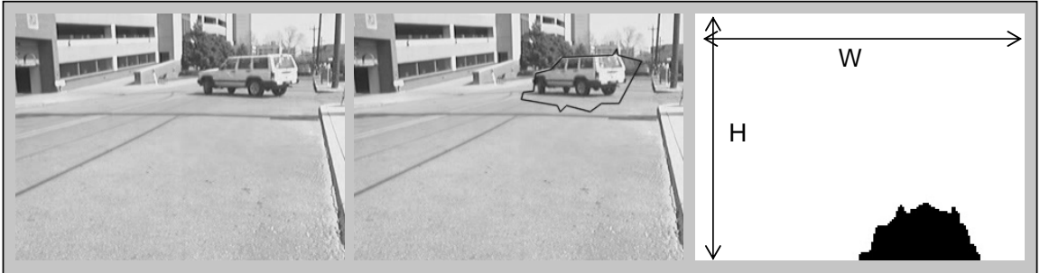
Figure 13: Video detection. The frame on the left shows the input image, the frame in the middle shows the foreground and the frame on the right shows the video detection function.
