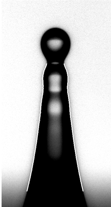
Figure 2.4. Free surface profile (white line) extracted from the original digital picture.
