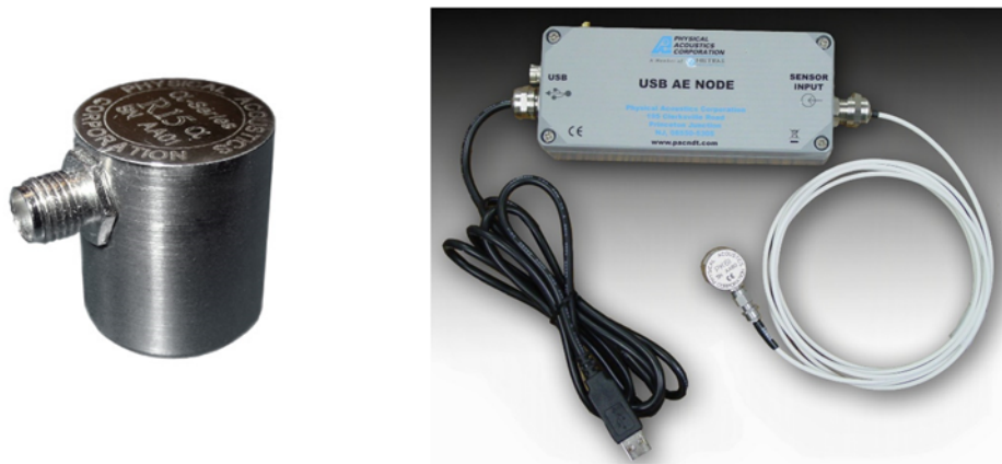
Figure B.6. R15- \alpha type sensor (left) and 1283 USB AE Node (right).
