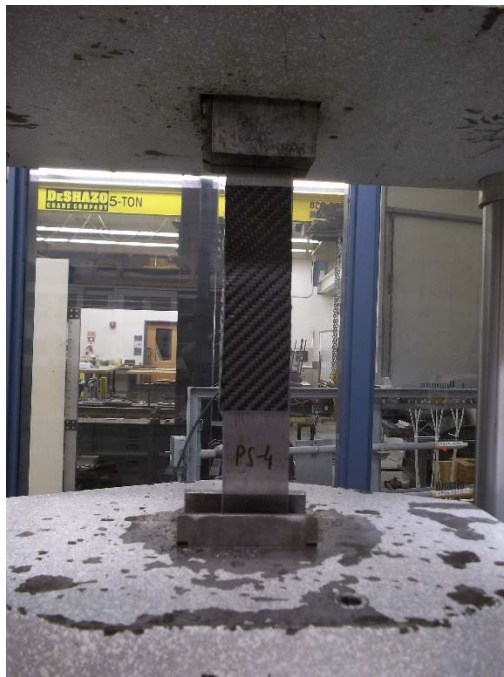
(a) Shear test specimen
