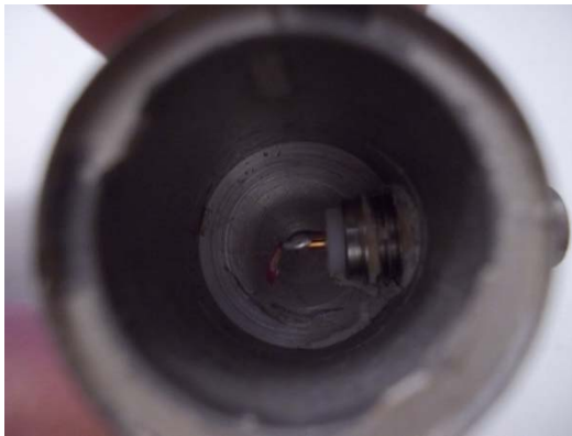
(c) After epoxy removal in base
