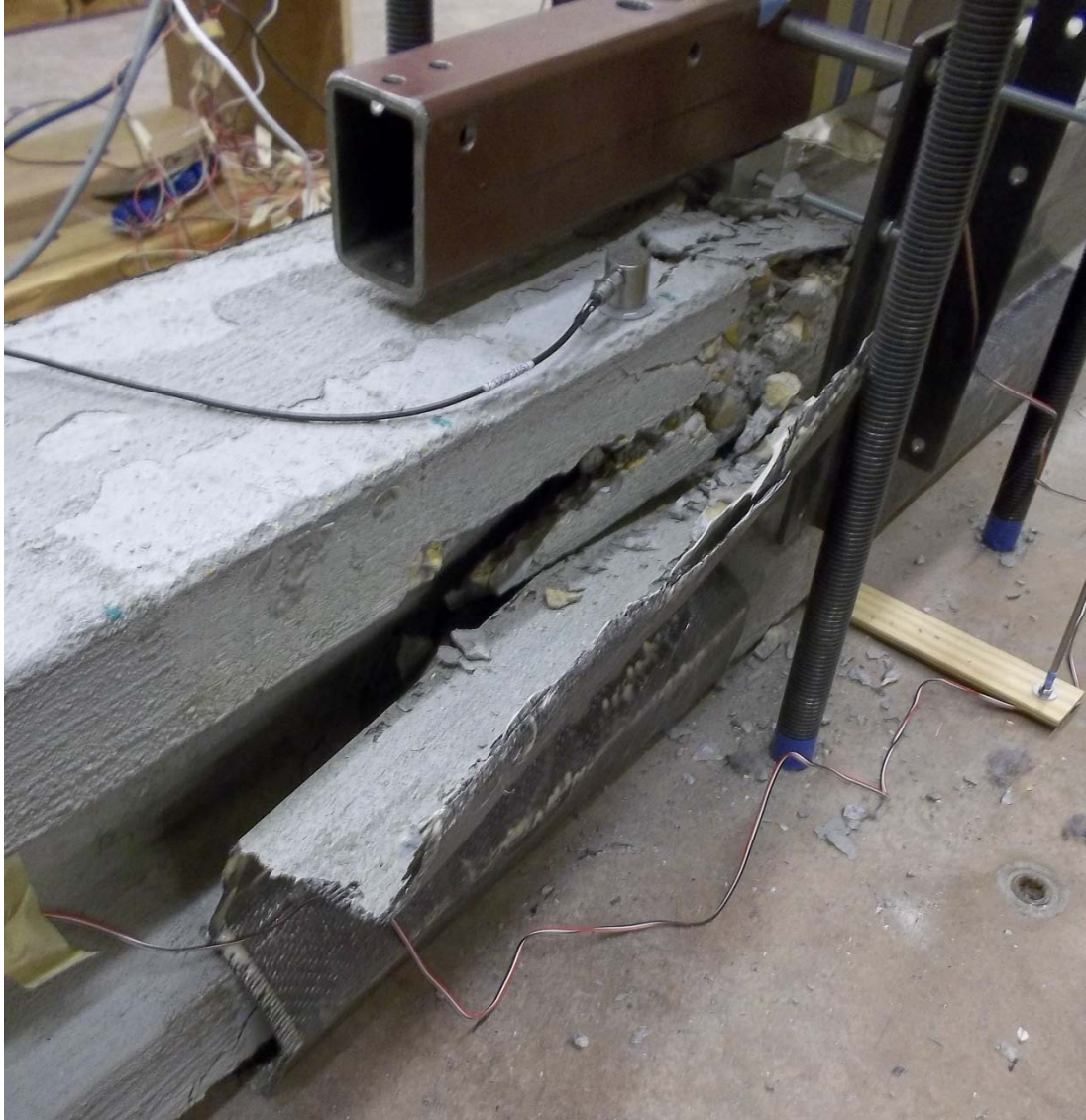
Figure 3.4.24. PSCB3 ultimately failed in shear in combination with concrete crushing on top and debonding.
