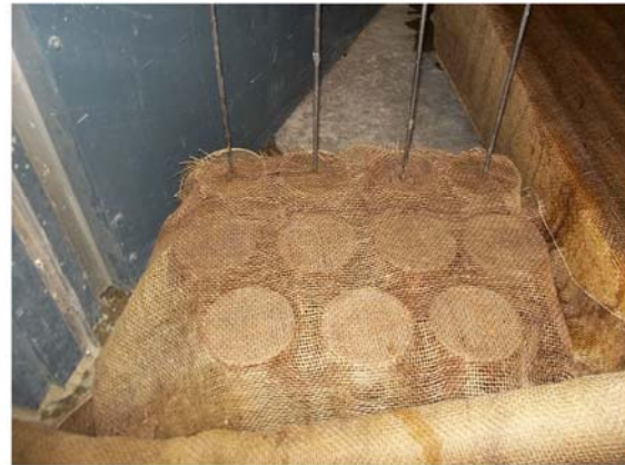
(b) Test cylinder with burlap cover
