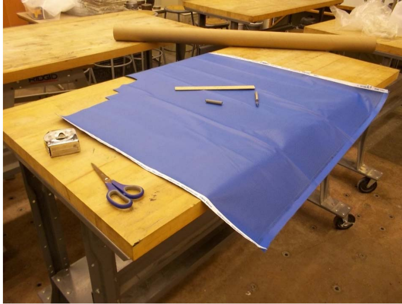
Figure G.4. Tools used to cut Fibreglast Prepreg 3K FRP Composite.
