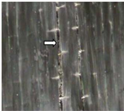
Figure 3.4.22. Cracking of the U-jacket composite patch of PSCB1 [65].
