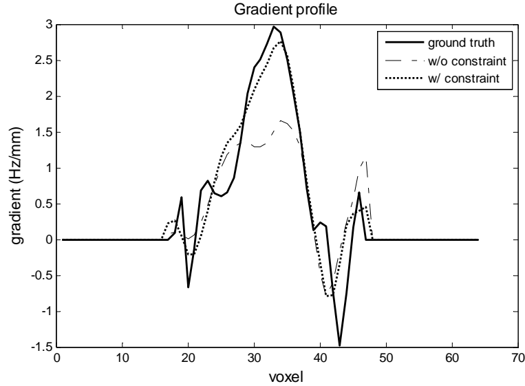
Figure 40. Gradient profile (indicated by a red line in Figure 39). The solid line is the true gradient of the distortion field. The dashed line is the gradient from the estimated distortion with standard non-rigid registration. The dotted line is the gradient from the estimated distortion field with the phase-gradient constraint. As it shows, the gradients of the distortion field computed with the new constraint is closer to that of the ground truth than the standard non-rigid registration without phase information.
